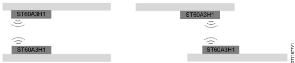
Figure 29. Supported ST60A3H1 180° relative orientations
