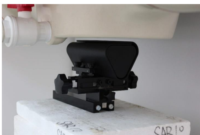
Front edge with Triangle at 5 mm
