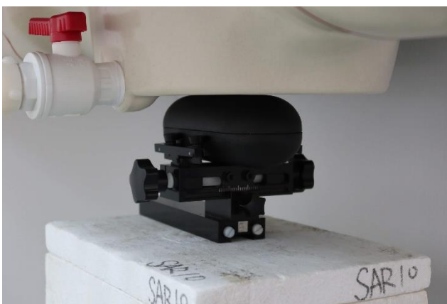
Bottom edge at 0° with Clamshell at 0 mm
