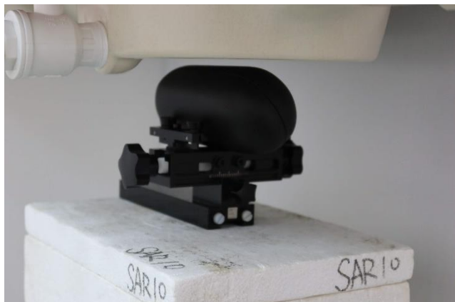
Bottom edge at 45° with Clamshell at 5 mm
