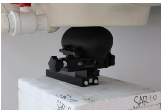
Bottom edge at -45° with Clamshell at 0 mm
