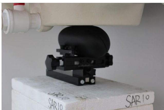
Bottom edge at 45° with Clamshell at 0 mm
