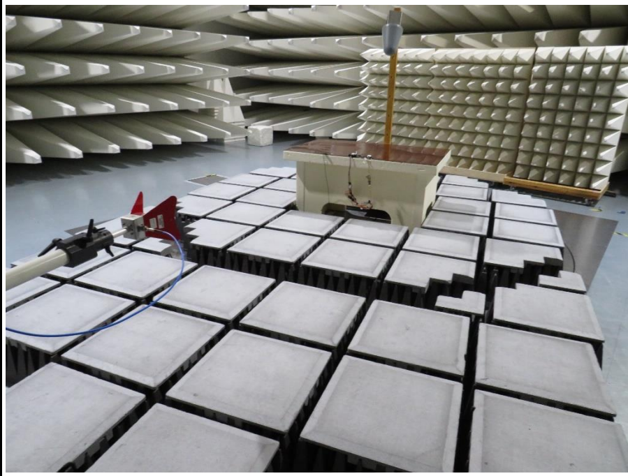
Test setup up above 1 GHz horizontal polarisation
