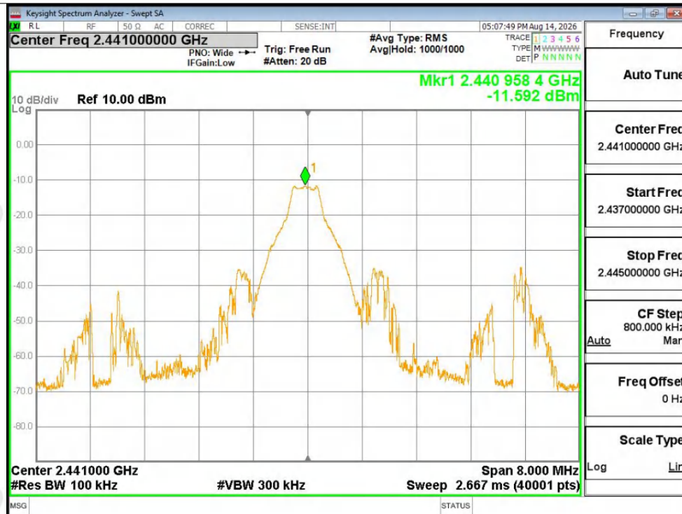
Tx. Spurious NVNT 1-DH5 2441MHz Ant1 Ref
