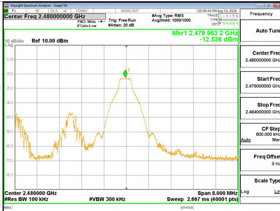
Tx. Spurious NVNT 1-DH5 2480MHz Ant1 Ref
