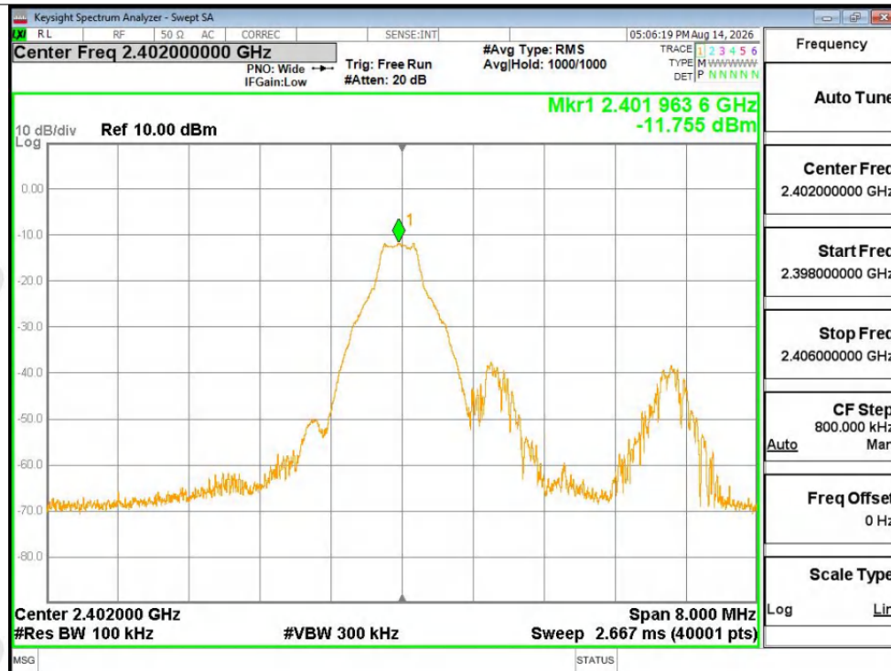
Tx. Spurious NVNT 1-DH5 2402MHz Ant1 Ref
