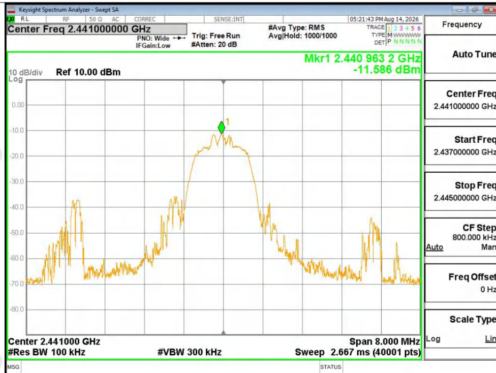
Tx. Spurious NVNT 2-DH5 2441MHz Ant1 Ref
