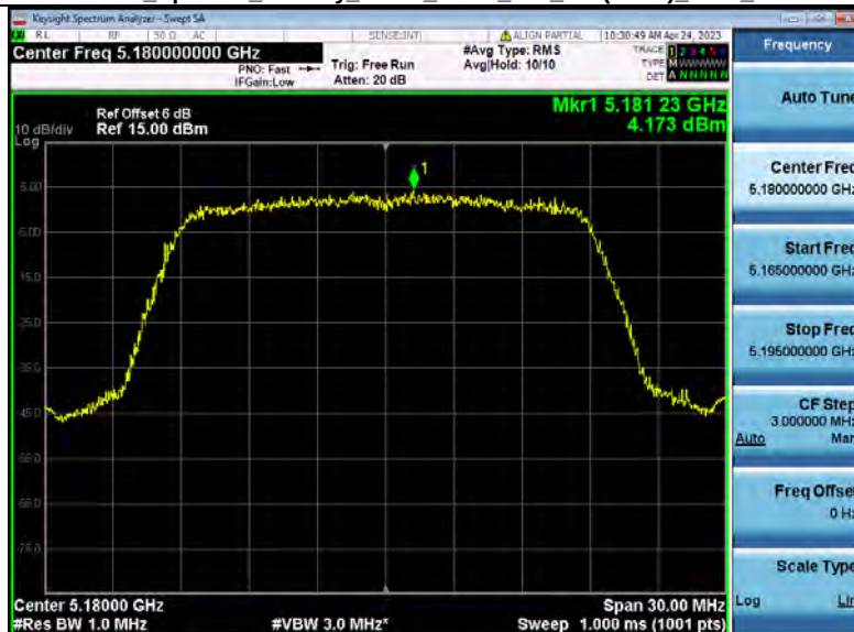
Power Spectral Density NVNT_ANT3_802_11n(HT20)_5180_20M
