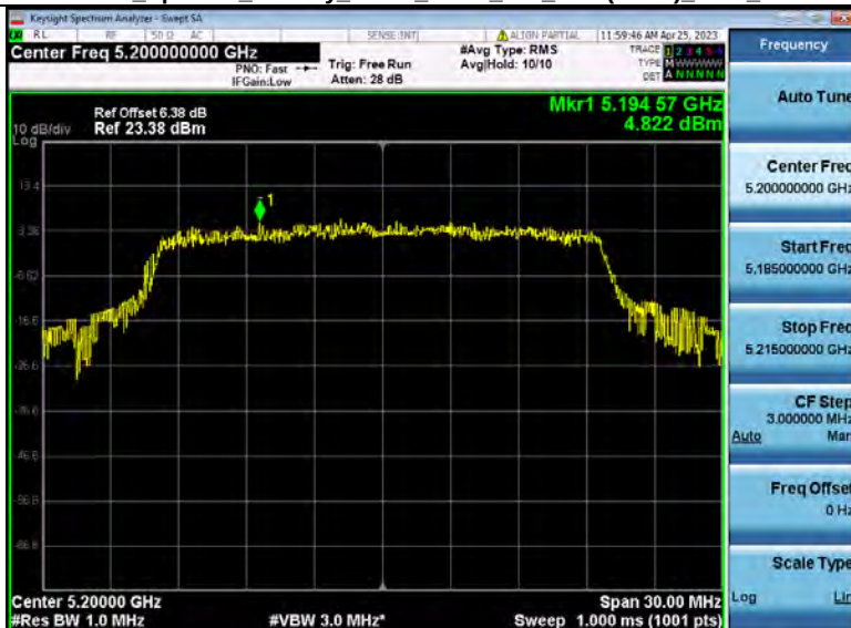
Power Spectral Density NVNT_ANT4_802_11ax(HE20)_5200_20M
