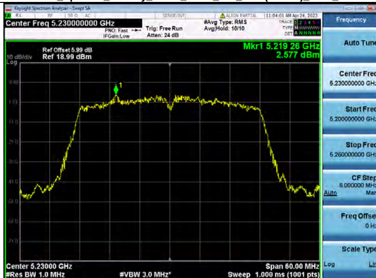
Power Spectral Density_NVNT_ANT4_802_11ac(VHT40)_5230_40M
