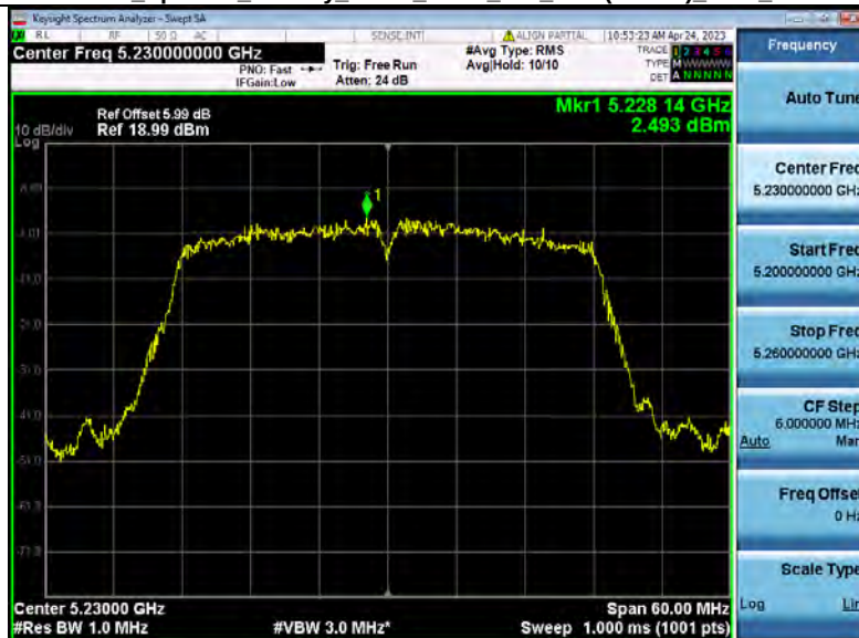
Power Spectral Density_NVNT_ANT3_802_11ac(VHT40)_5230_40M
