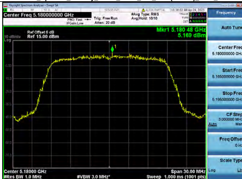
Power Spectral Density NVNT_ANT3_802_11ac(VHT20)_5180_20M
