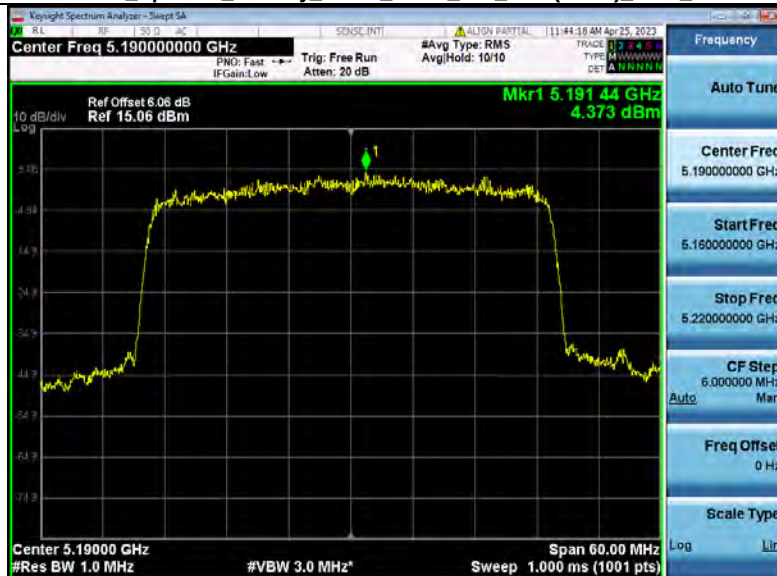
Power Spectral Density_NVNT_ANT3_802_11ax(HE40)_5190_40M
