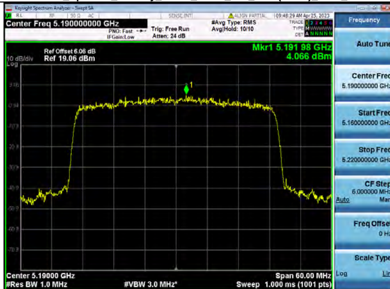
Power Spectral Density_NVNT_ANT2_802_11ax(HE40)_5190_40M
