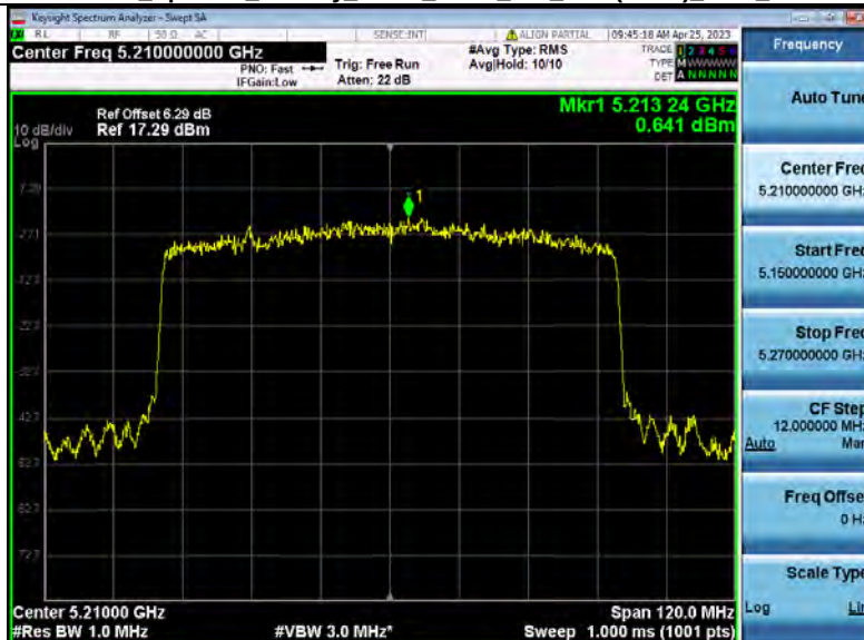
Power Spectral Density NVNT_ANT2_802_11ax(HE80)_5210_80M
