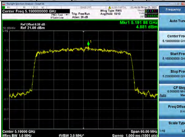
Power Spectral Density_NVNT_ANT4_802_11ax(HE40)_5190_40M
