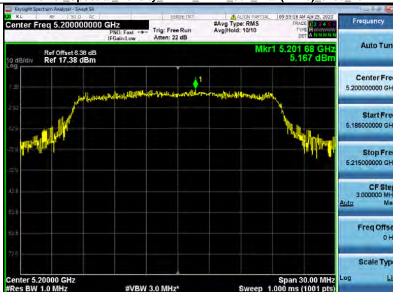
Power Spectral Density NVNT_ANT2_802_11ax(HE20)_5200_20M
