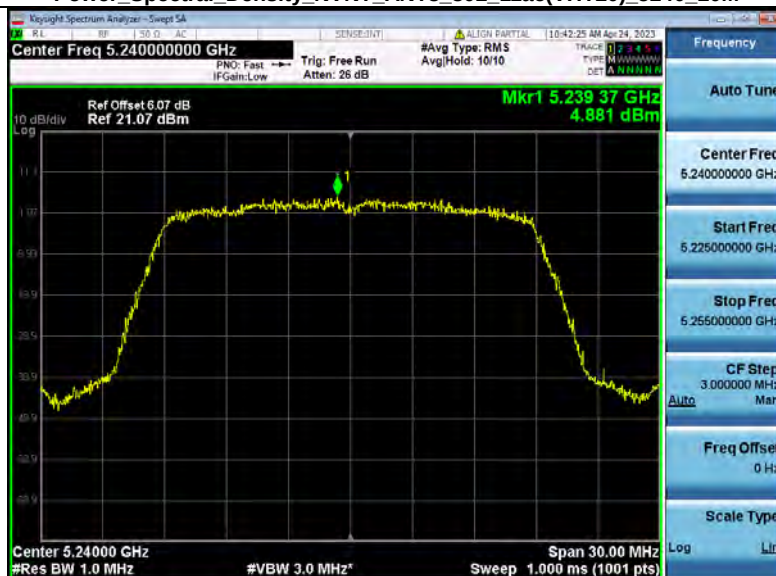
Power Spectral Density NVNT_ANT3_802_11ac(VHT20)_5240_20M
