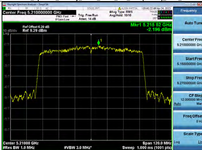
Power Spectral Density NVNT_ANT2_802_11ax(HE80)_5210_80M
