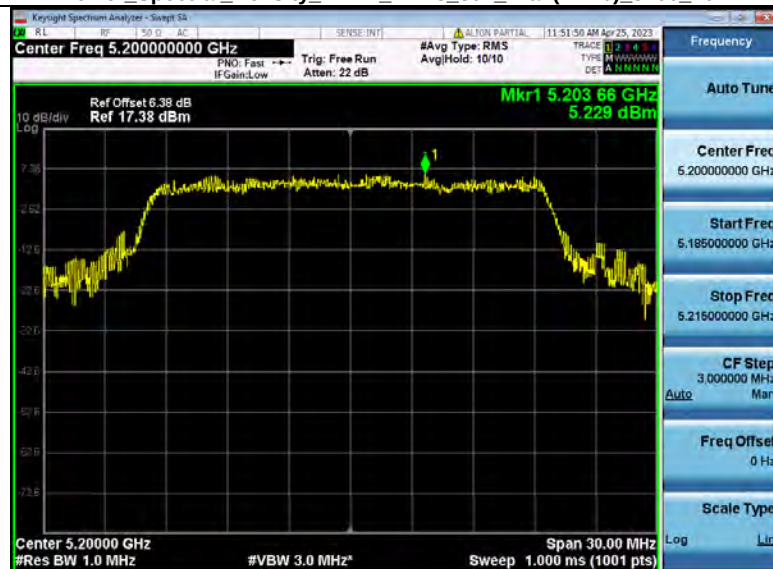
Power Spectral Density NVNT_ANT3_802_11ax(HE20)_5200_20M
