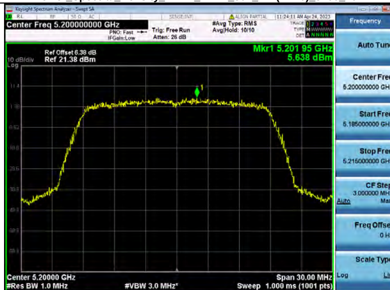
Power Spectral Density NVNT_ANT4_802_11n(HT20)_5200_20M
