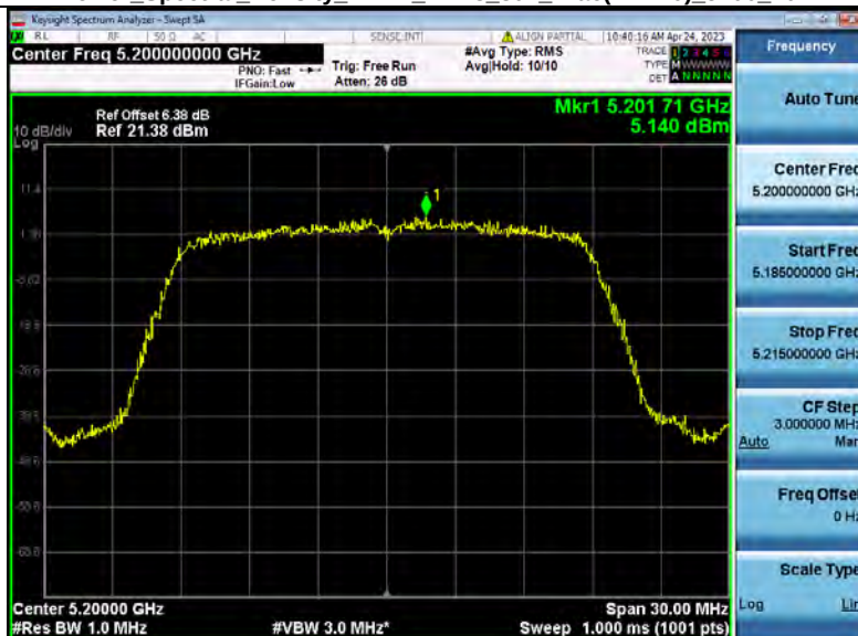
Power Spectral Density NVNT_ANT3_802_11ac(VHT20)_5200_20M
