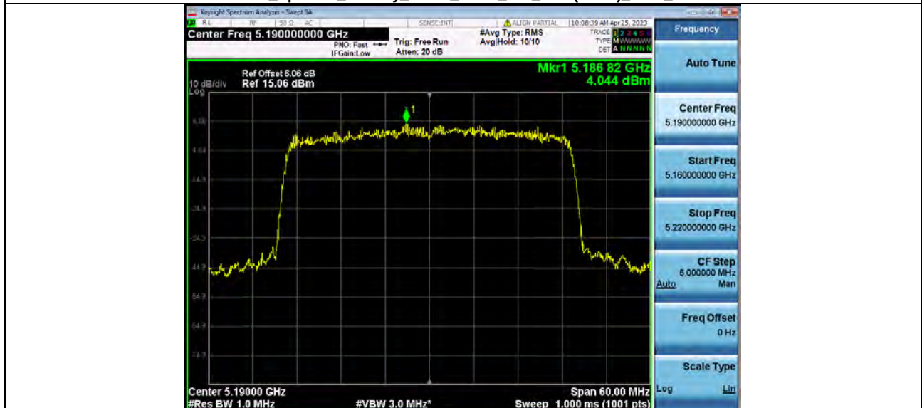
Power Spectral Density NVNT_ANT1_802_11ax(HE40)_5190_40M
