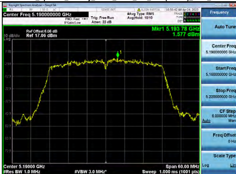
Power Spectral Density NVNT_ANT3_802_11ac(VHT40)_5190_40M
