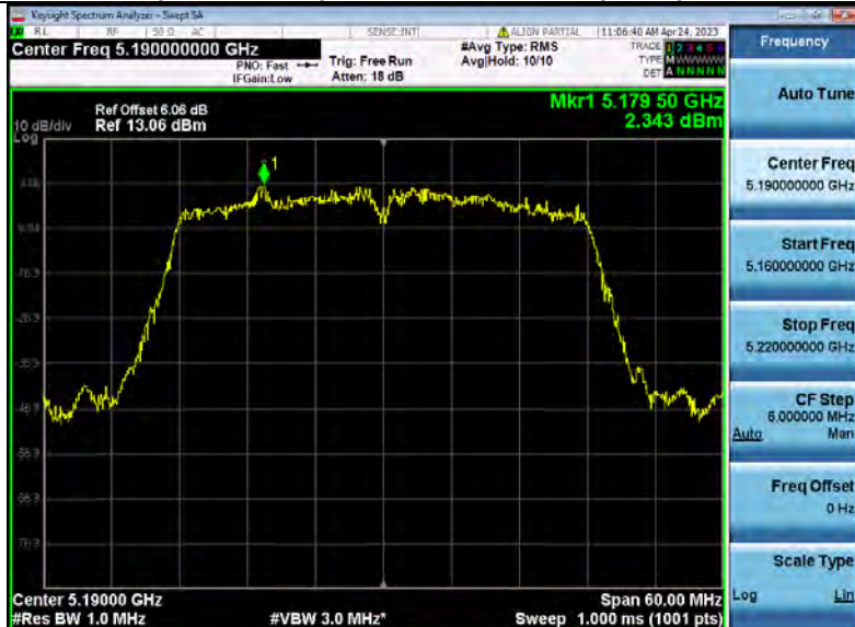
Power Spectral Density NVNT_ANT4_802_11ac(VHT40)_5190_40M
