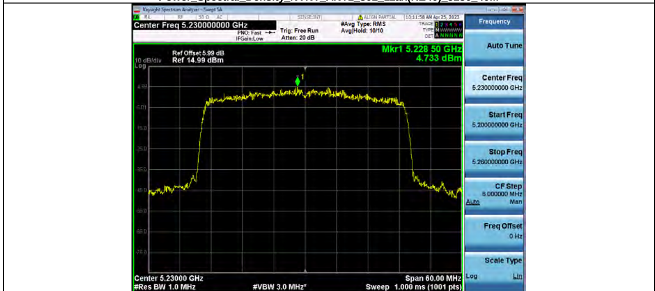
Power Spectral Density NVNT_ANT1_802_11ax(HE40)_5230_40M
