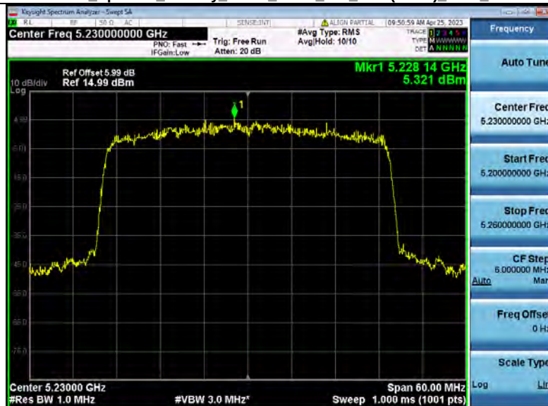
Power Spectral Density_NVNT_ANT2_802_11ax(HE40)_5230_40M
