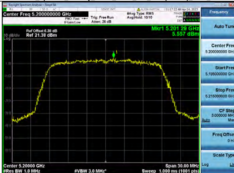
Power Spectral Density NVNT_ANT4_802_11ac(VHT20)_5200_20M
