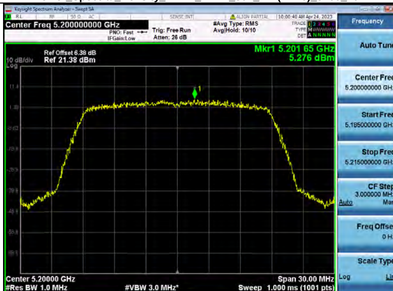
Power Spectral Density NVNT_ANT2_802_11n(HT20)_5200_20M
