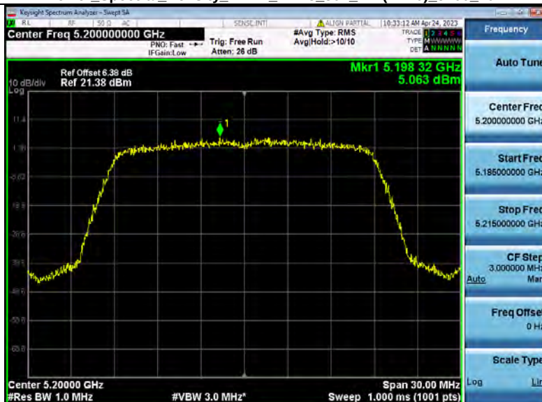
Power Spectral Density NVNT_ANT3_802_11n(HT20)_5200_20M
