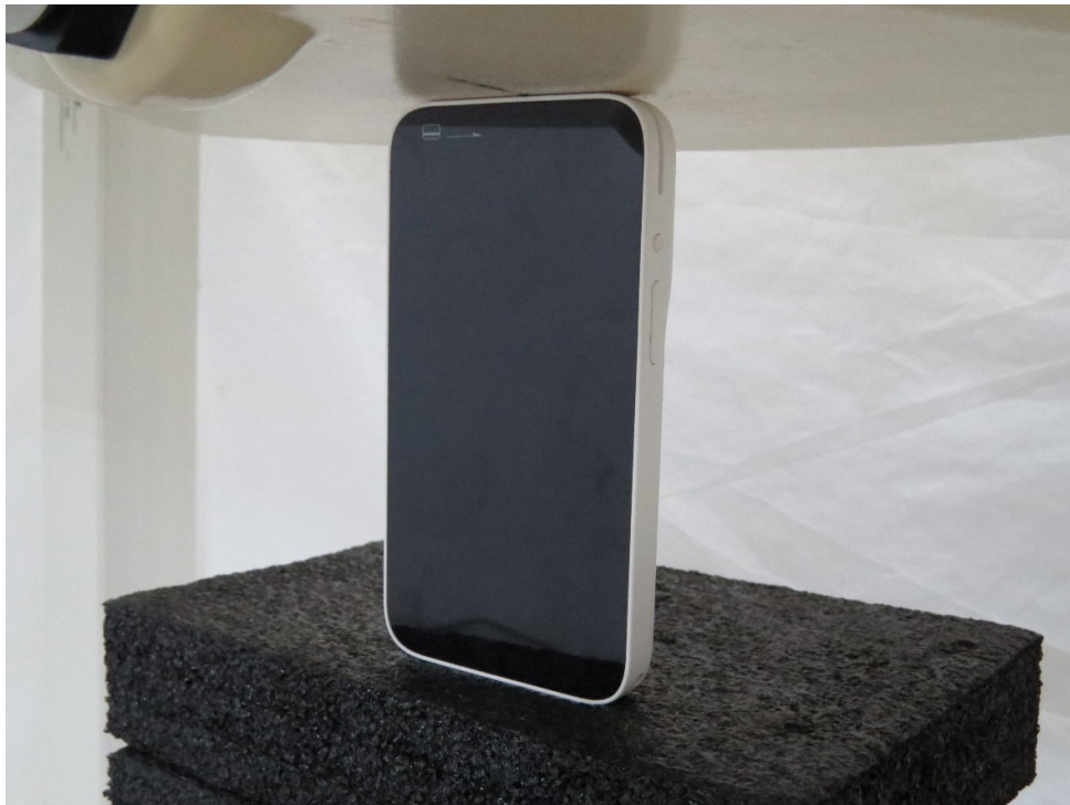
Picture 10: Top Edge, the distance from EUT to the bottom of the Phantom is 0mm
