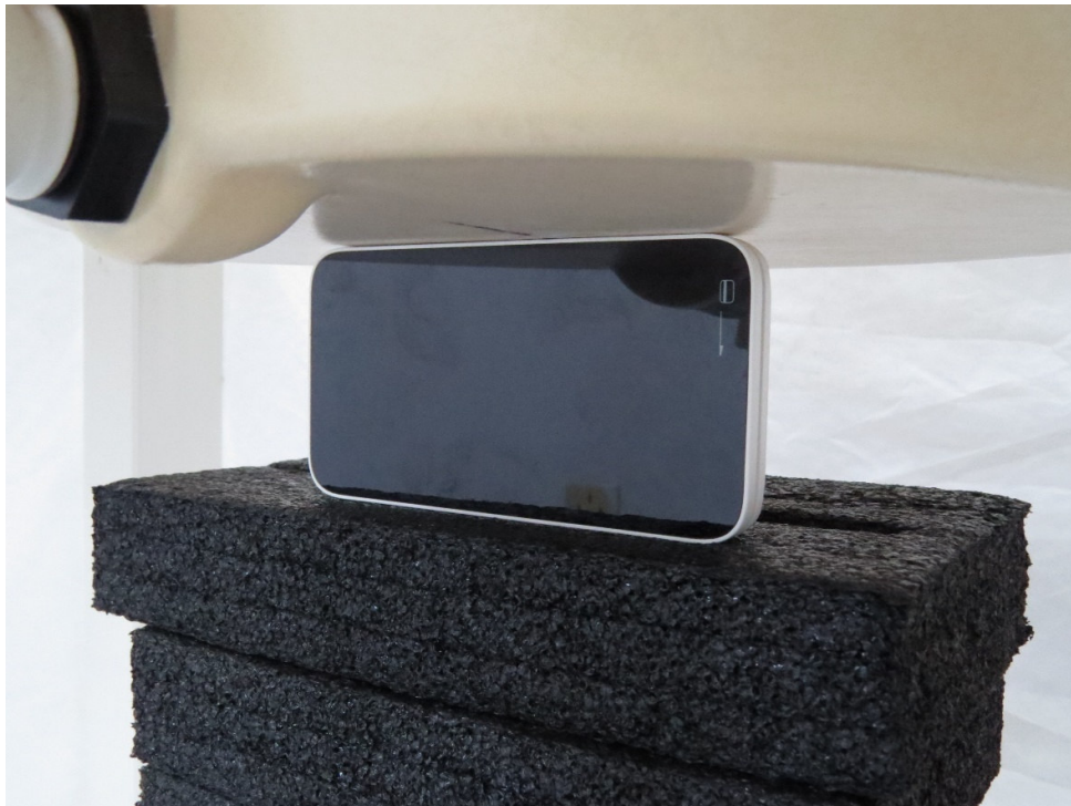
Picture 8: Left Edge, the distance from EUT to the bottom of the Phantom is 0mm
