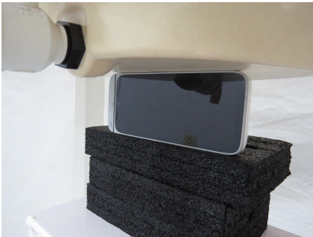
Picture 9: Antenna 0 and Antenna 2 Right Edge, the distance from EUT to the bottom of the Phantom is 0mm
