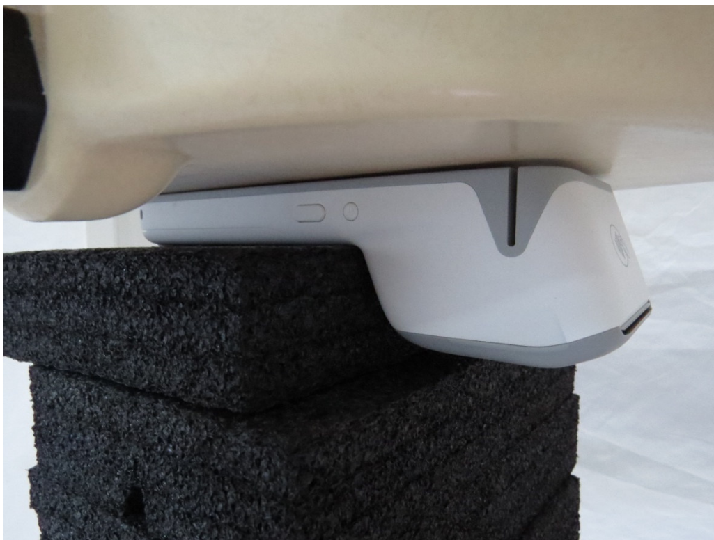
Picture 7: Antenna 0 and Antenna 2 Front Side, the distance from EUT to the bottom of the Phantom is 0mm
