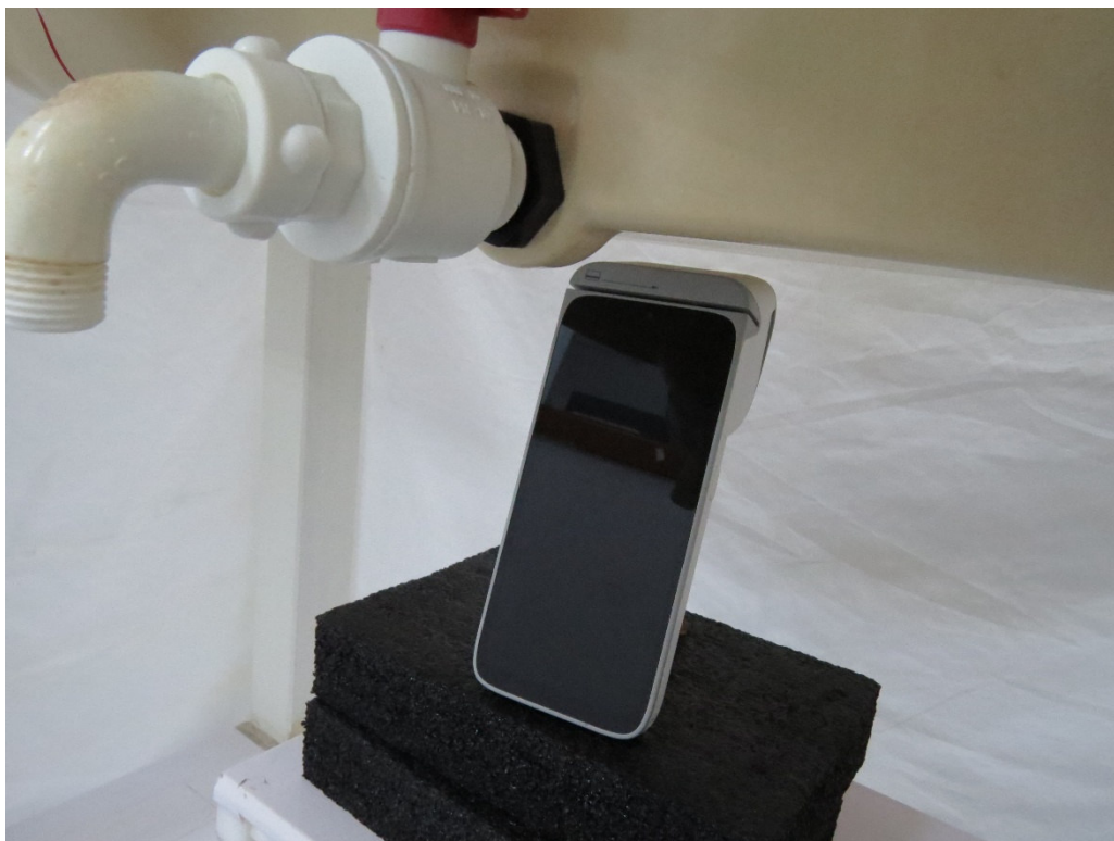
Picture 5: Antenna 0 and Antenna 2 Top Edge, the distance from EUT to the bottom of the Phantom is 10mm
