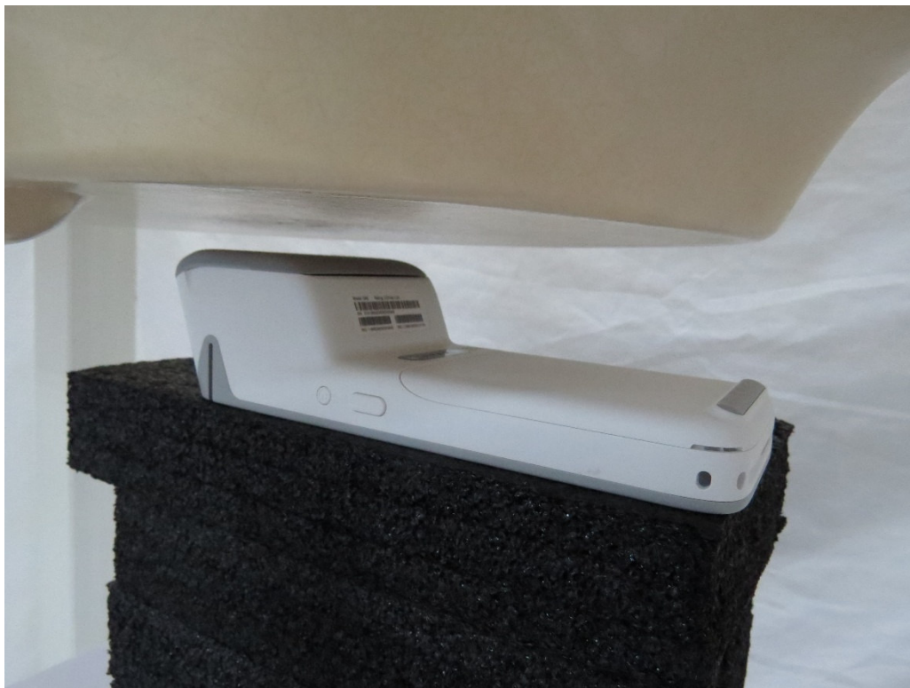
Picture 1: Antenna 0 Back Side, the distance from EUT to the bottom of the Phantom is 10mm
