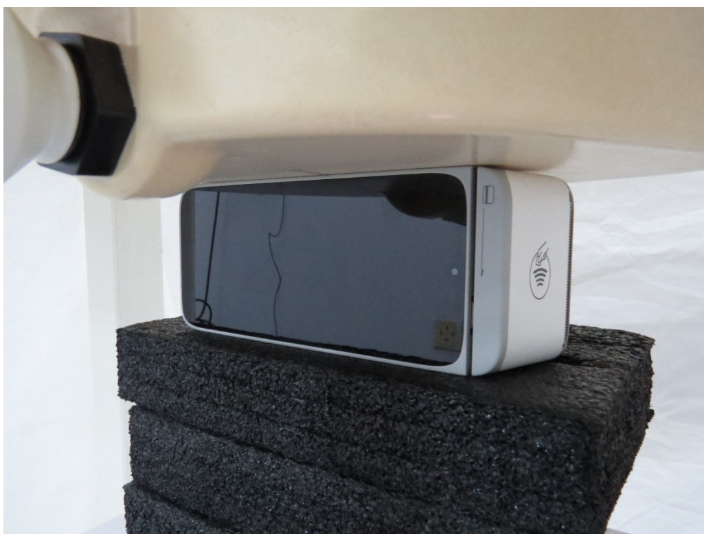
Picture 8: Antenna 0 and Antenna 2 Left Edge, the distance from EUT to the bottom of the Phantom is 0mm
