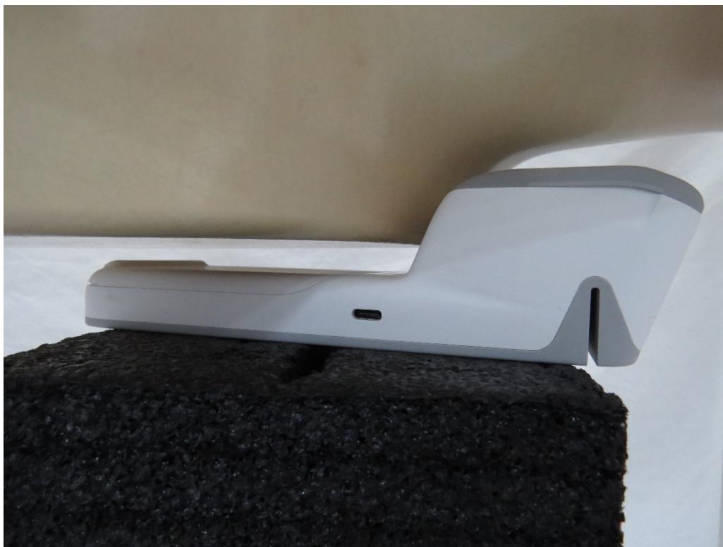
Picture 2: Antenna 2 Back Side, the distance from EUT to the bottom of the Phantom is 10mm
