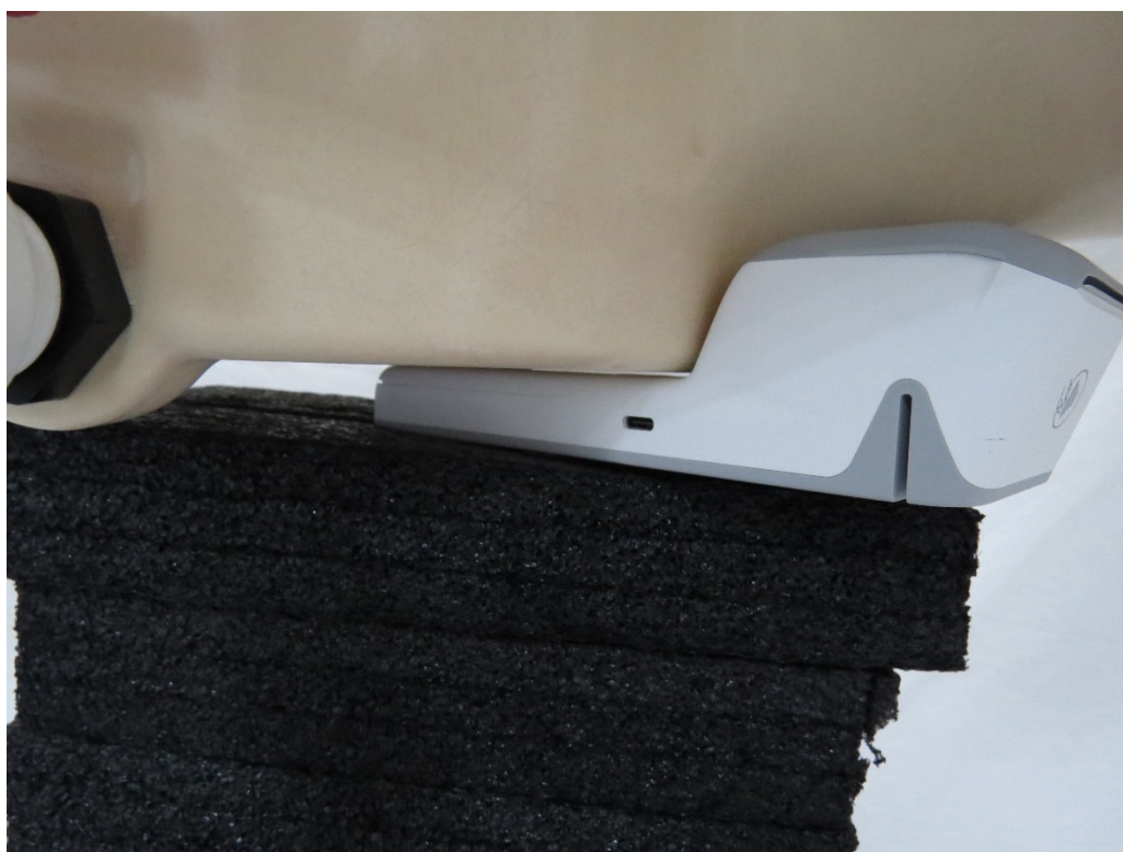
Picture 6: Antenna 2 Back Side, the distance from EUT to the bottom of the Phantom is 0mm
