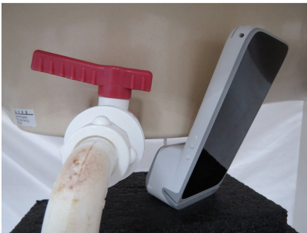
Picture 1: Antenna 0 Back Side2, the distance from EUT to the bottom of the Phantom is 10mm
