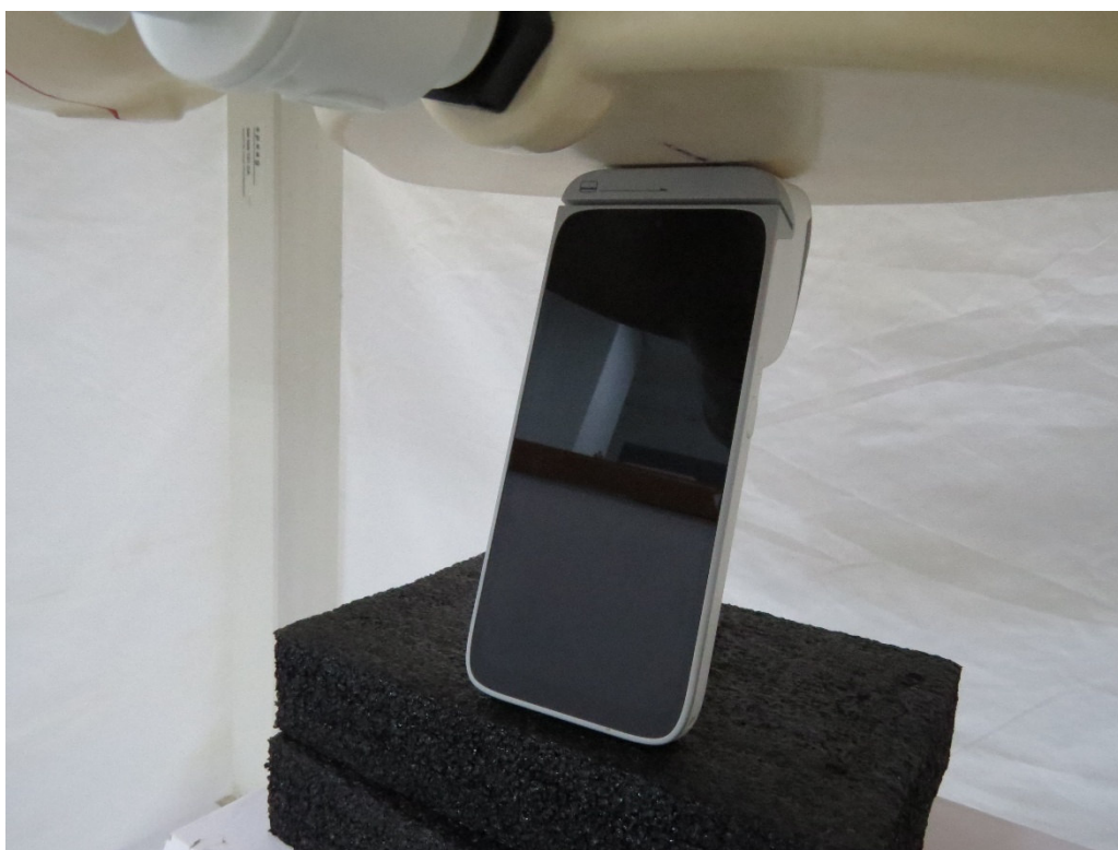
Picture 10: Antenna 0 and Antenna 2 Top Edge, the distance from EUT to the bottom of the Phantom is 0mm
