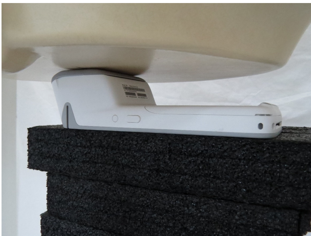
Picture 6: Antenna 0 Back Side, the distance from EUT to the bottom of the Phantom is 0mm
