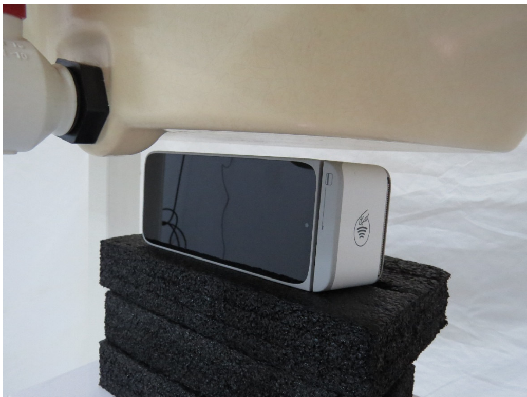
Picture 3: Antenna 0 and Antenna 2 Left Edge, the distance from EUT to the bottom of the Phantom is 10mm
