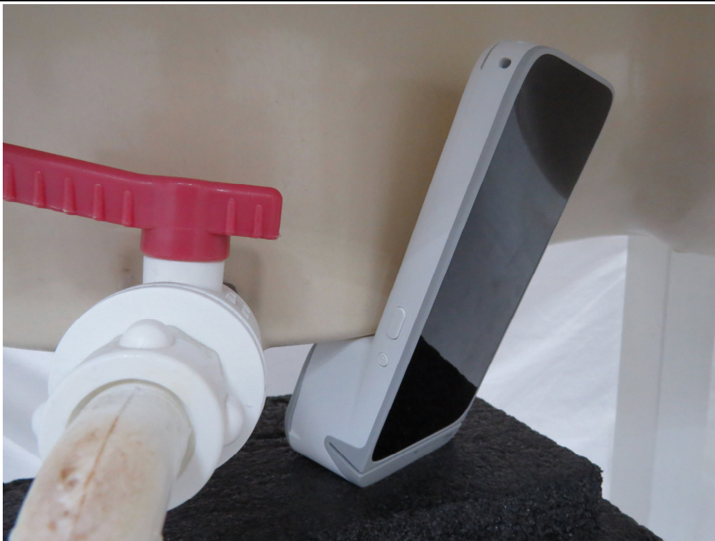
Picture 6: Antenna 0 Back Side2, the distance from EUT to the bottom of the Phantom is 0mm
