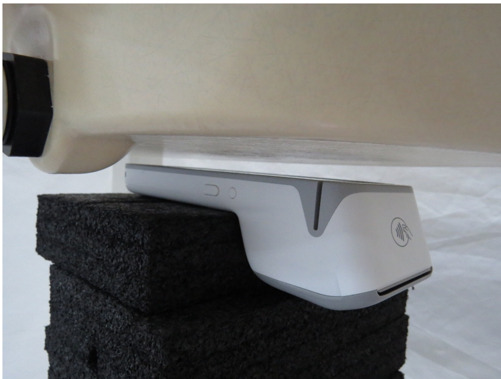
Picture 2: Antenna 0 and Antenna 2 Front Side, the distance from EUT to the bottom of the Phantom is 10mm
