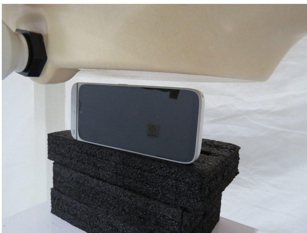
Picture 4: Antenna 0 and Antenna 2 Right Edge, the distance from EUT to the bottom of the Phantom is 10mm
