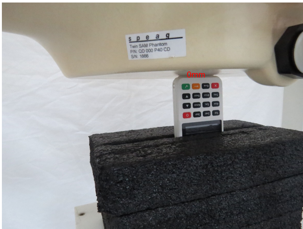
Picture 12: Bottom Edge, the distance from EUT to the bottom of the Phantom is 0mm
