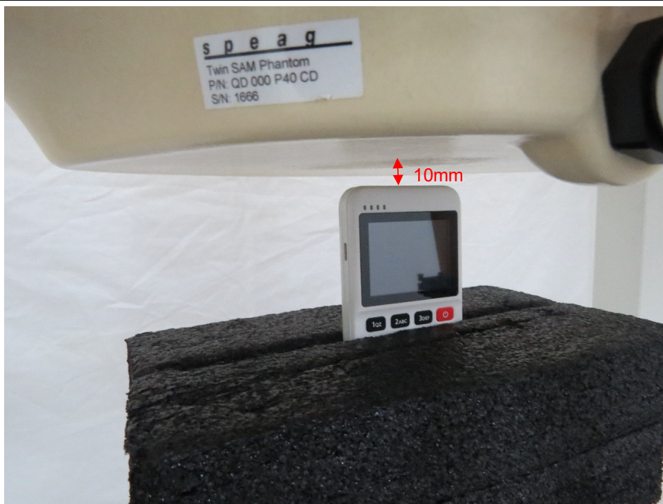
Picture 5: Top Edge, the distance from EUT to the bottom of the Phantom is 10mm
