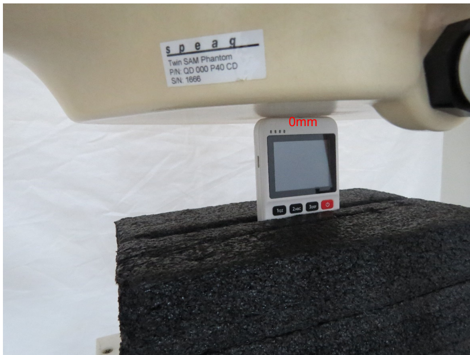
Picture 11: Top Edge, the distance from EUT to the bottom of the Phantom is 0mm
