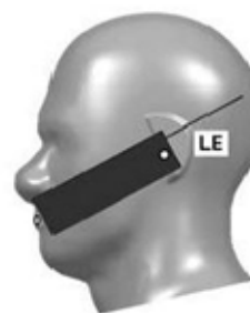
Picture17 Tilt position. The reference points for the right ear (RE), left ear (LE), and mouth (M), which define the Reference Plane for handset positioning, are indicated.
