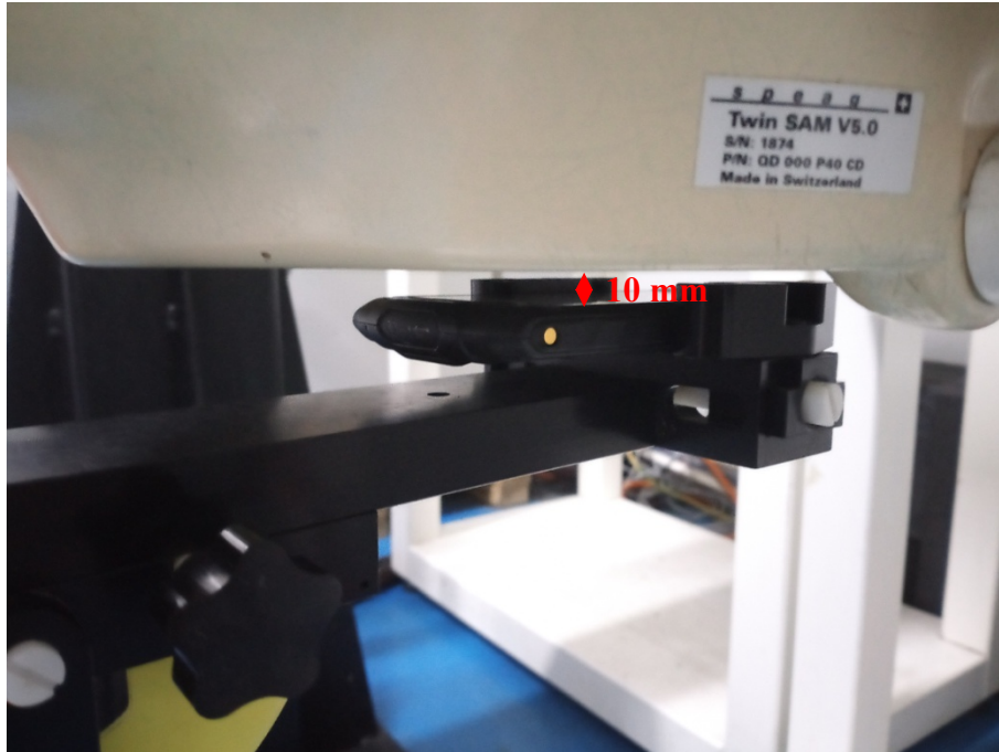
Body Front Setup Photo(10mm)
