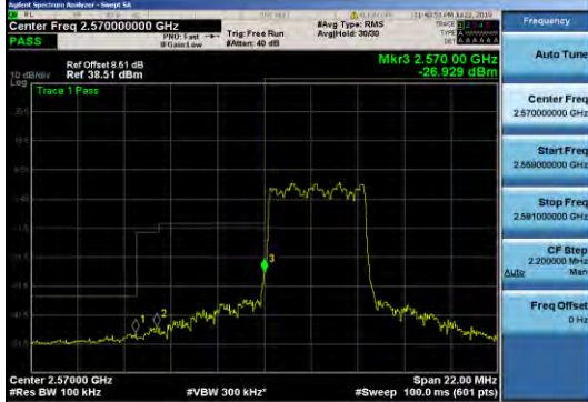
Band38 5MHz 16QAM 37775 25RB#0
