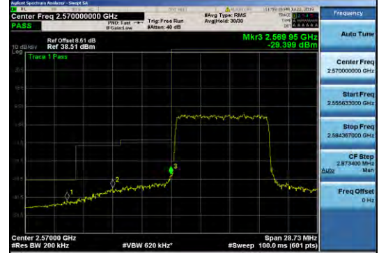
Band38 10MHz QPSK 37800 50RB#0
