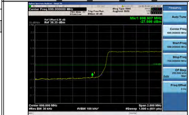
Band12 3MHz QPSK 23025 15RB#0
