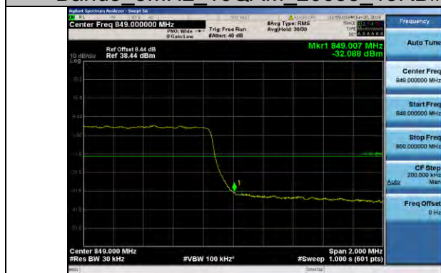
Band5 3MHz 16QAM 20635 15RB#0
