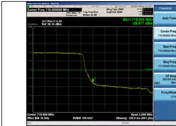
Band12 1.4MHz 16QAM 23017 1RB#0
