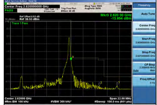
Band38 5MHz 16QAM 38225 25RB#0
