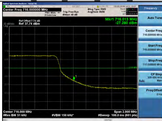
Band17 5MHz QPSK 23825 25RB#0
