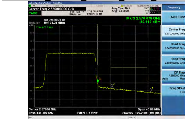
Band7 20MHz 16QAM 21350 100RB#0
