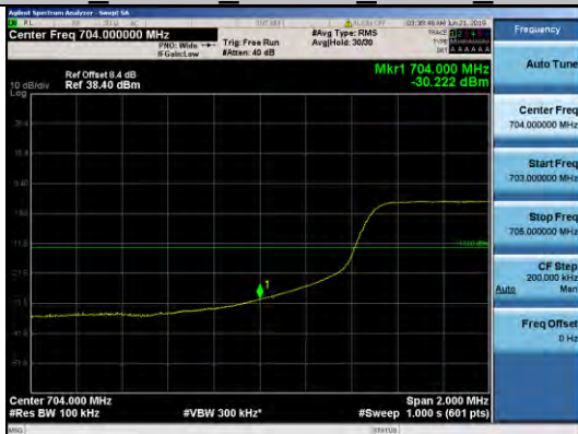
Band17 10MHz 16QAM 23780 50RB#0
