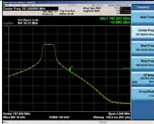
Band13 5MHz QPSK 23255 25RB#0
