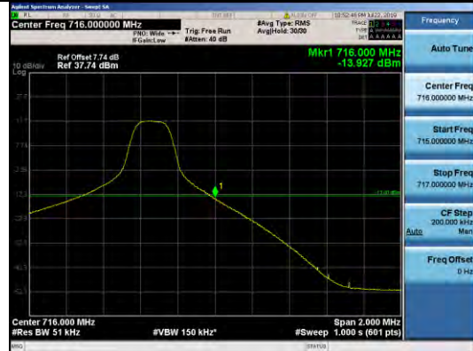
Band12 5MHz QPSK 23155 25RB#0
