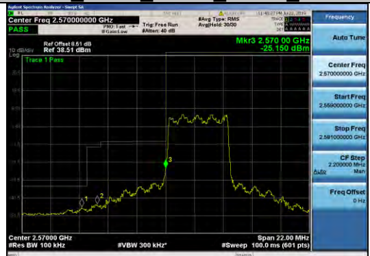
Band38 5MHz QPSK 37775 25RB#0
