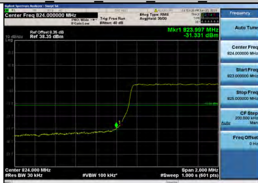
Band5 3MHz QPSK 20415 15RB#0
