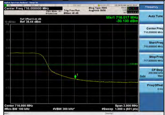
Band12 10MHz 16QAM 23130 50RB#0
