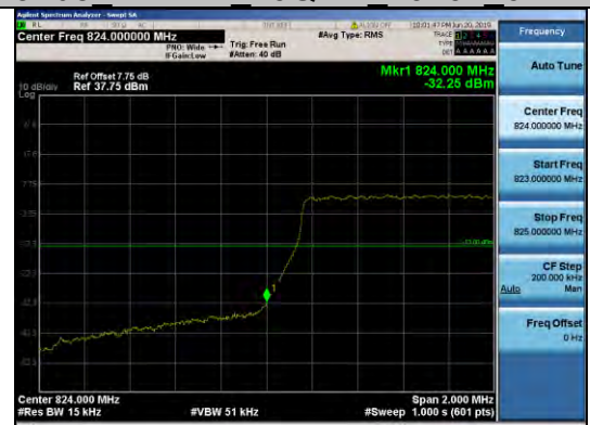
Band5 1.4MHz 16QAM 20407 6RB#0
