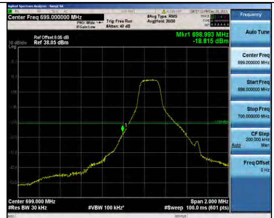
Band12 1.4MHz QPSK 23017 6RB#0
