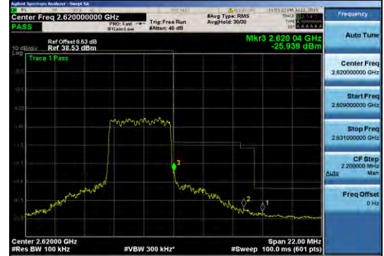
Band38 5MHz 16QAM 38225 25RB#0
