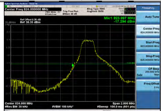
Band5 3MHz 16QAM 20415 15RB#0
