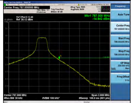
Band13 5MHz 16QAM 23255 25RB#0
