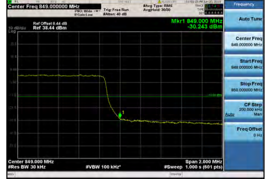
Band5 3MHz 16QAM 20415 1RB#0
