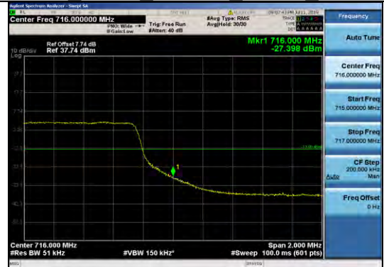
Band12 5MHz 16QAM 23155 25RB#0
