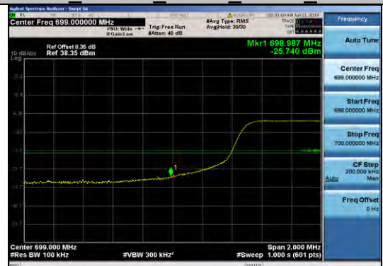
Band12 10MHz QPSK 23060 50RB#0
