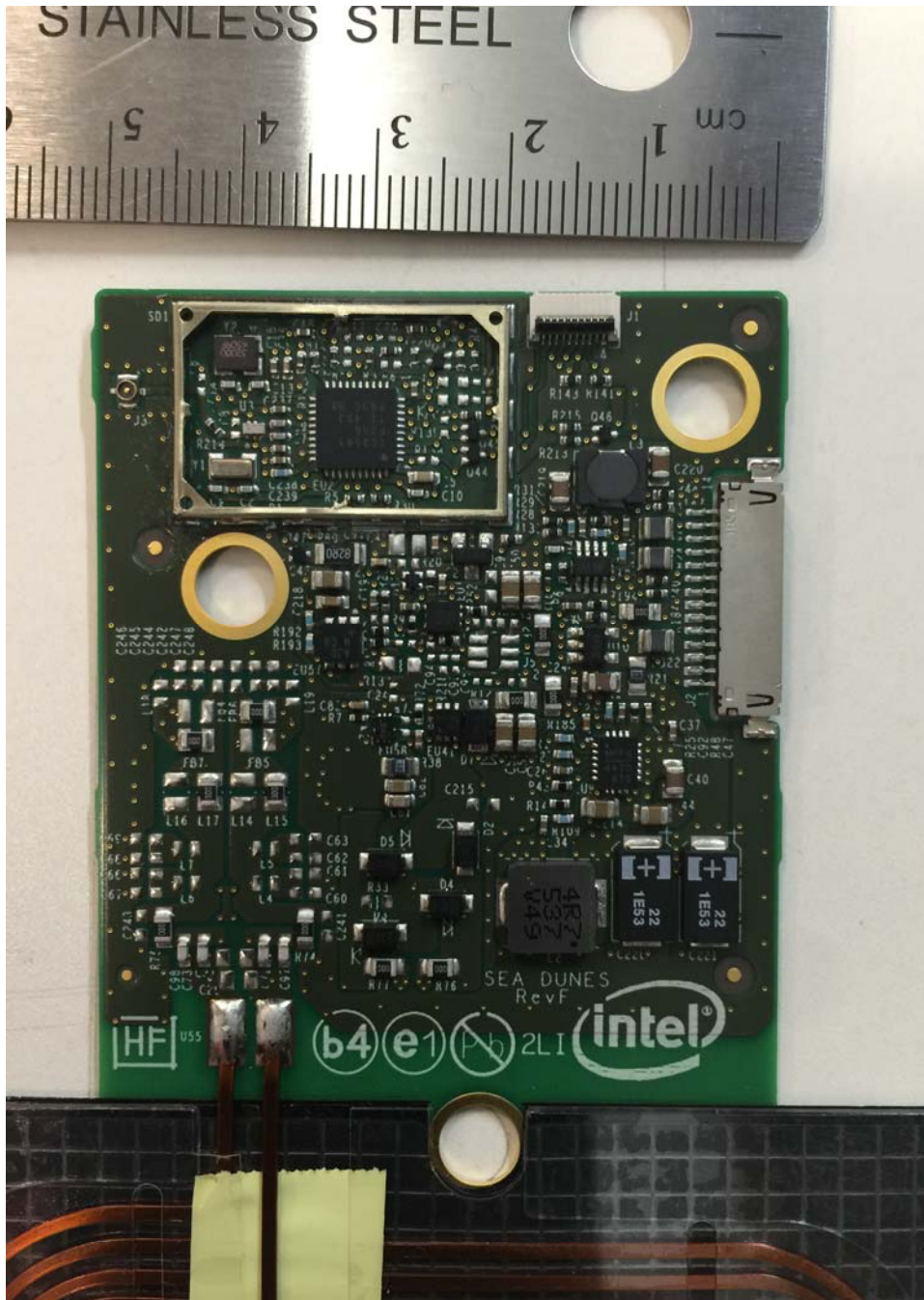
Top View of Board with shield over Bluetooth circuitry removed
