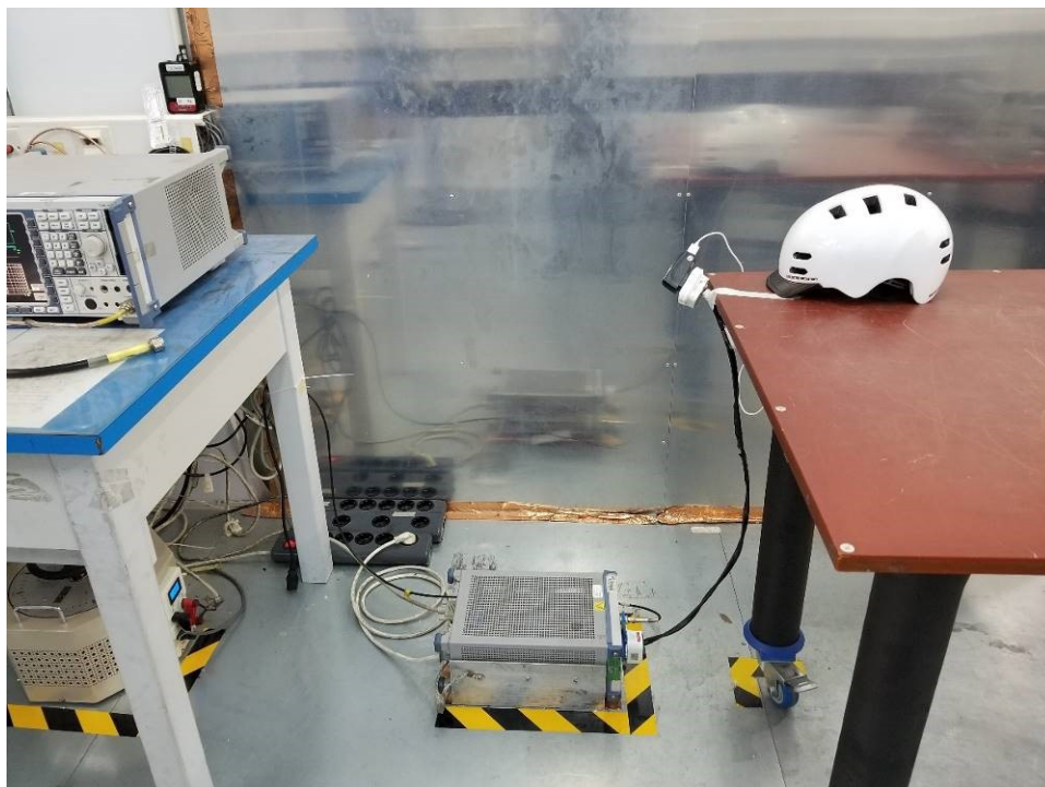
Photograph 5: Set-up for Conducted Emission on AC Mains
