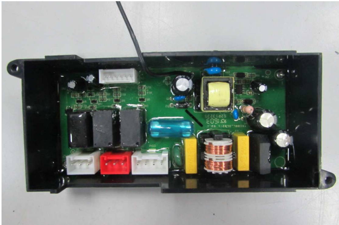
The power supply box inside view
