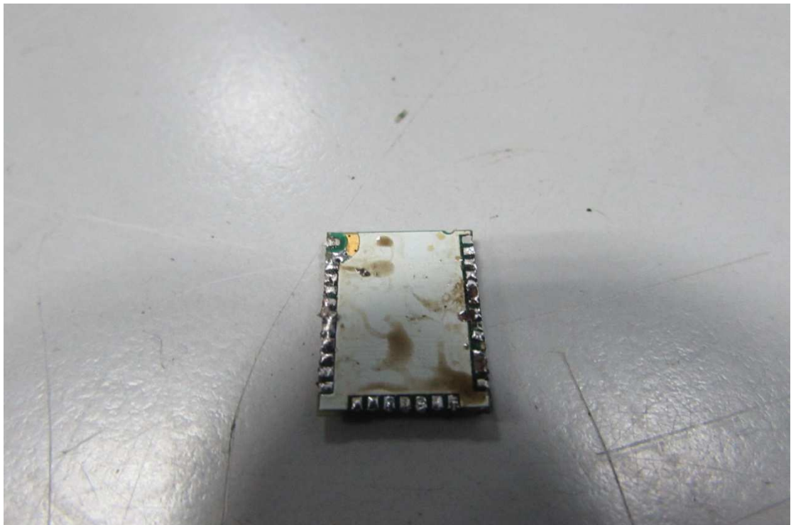
The Bluetooth module PCB view
