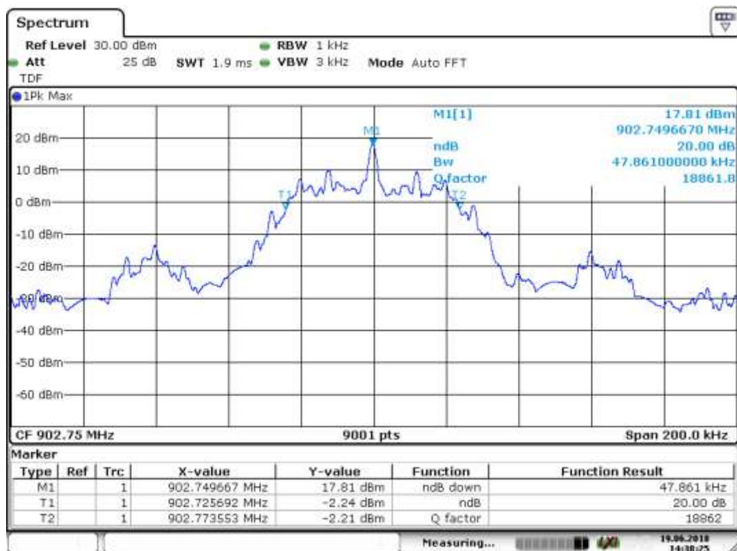
Figure 21. 20 dB channel BW channel LOW
