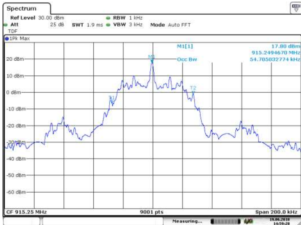
Figure 30. Mid channel 99% Occupied Power Bandwidth
