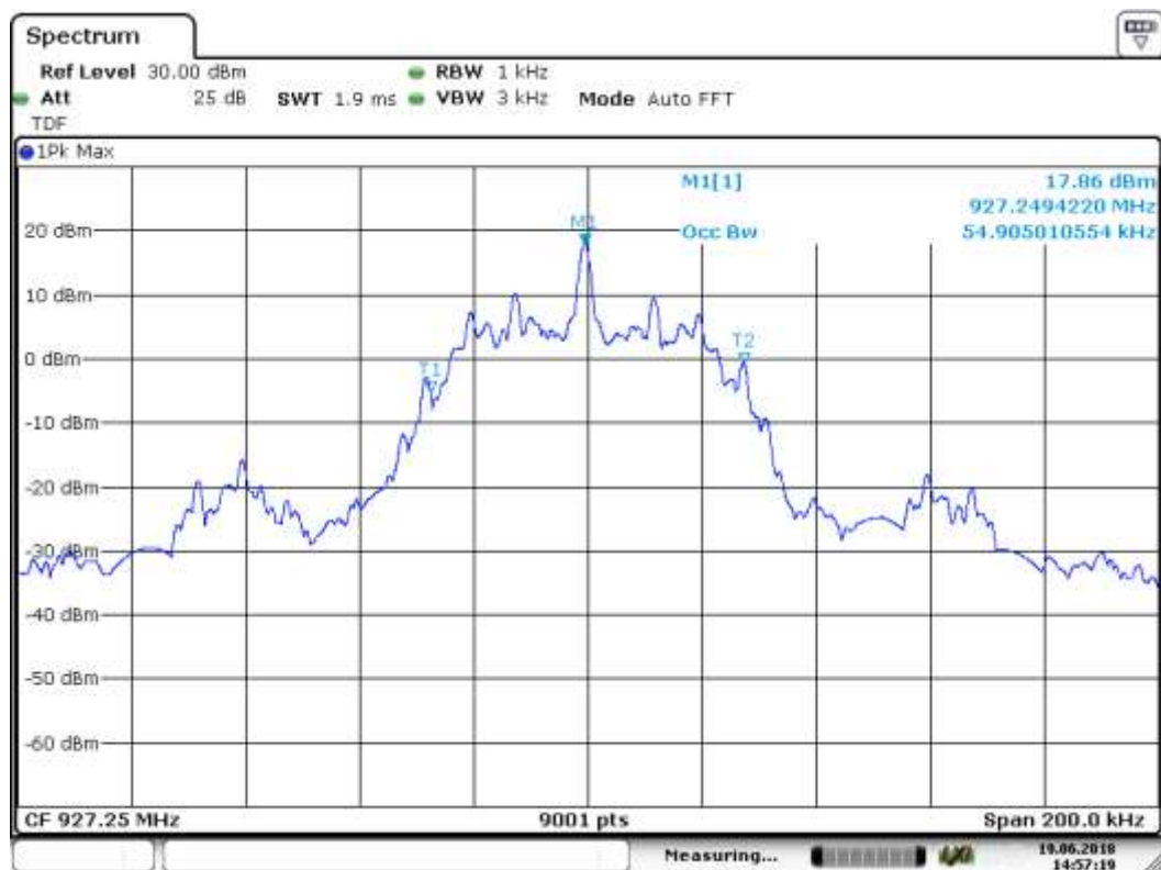
Figure 31. High channel 99% Occupied Power Bandwidth
