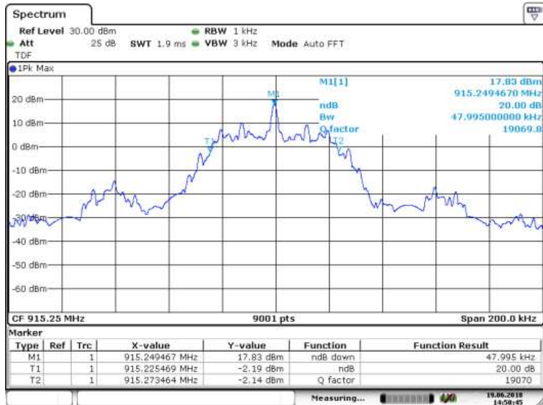
Figure 22. 20 dB channel BW channel MID
