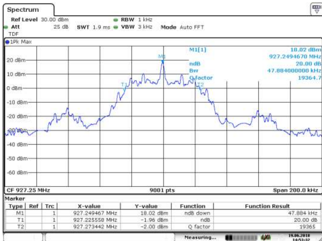
Figure 23. 20 dB channel BW channel HIGH
