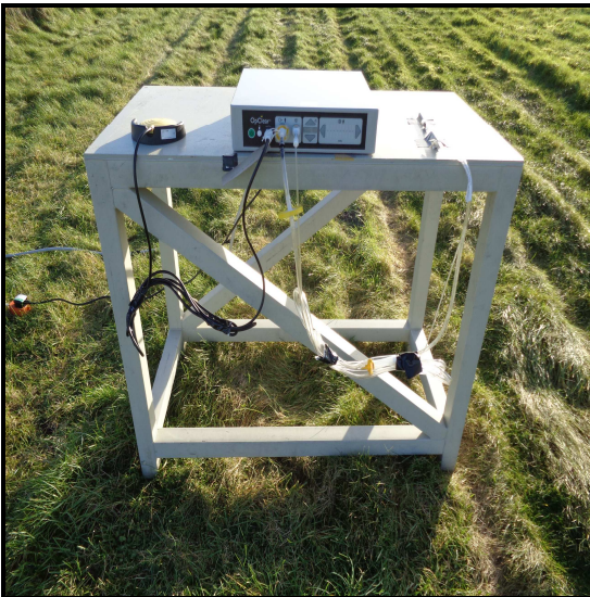
Set up for 300 metre measurements (EUT facing away from the mag loop antenna)
