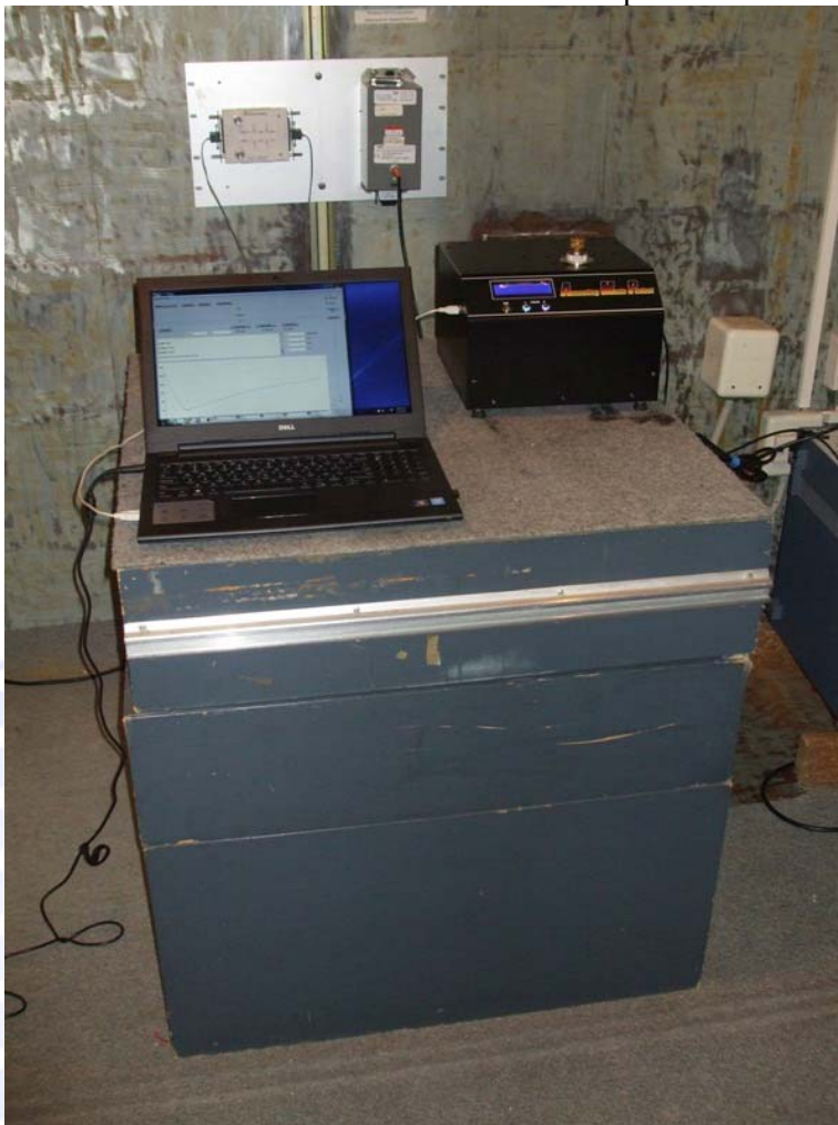
Conducted emissions test set up
