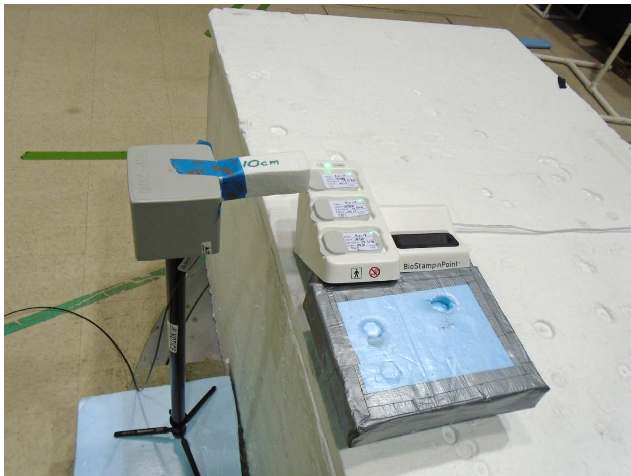
Figure 5: E-Field and H-Field – Right Side at 1% Charge on Battery Field Probe was placed 10 cm from the EUT for all pictures. The Field Probe used is an NARDA-EHP200A
