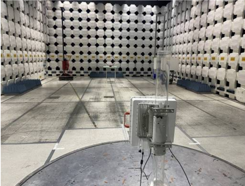
9 kHz-30 MHz Test Setup
