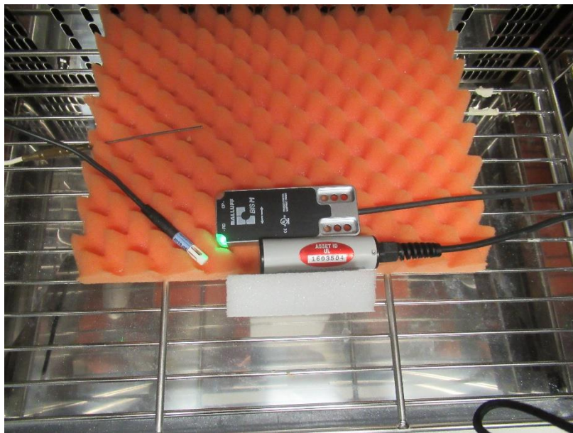
Photo 10 Bench test set up for (99% / 20 dB Bandwidth and Frequency Stability) (@ Ambient + Extreme Temperature, as required)
