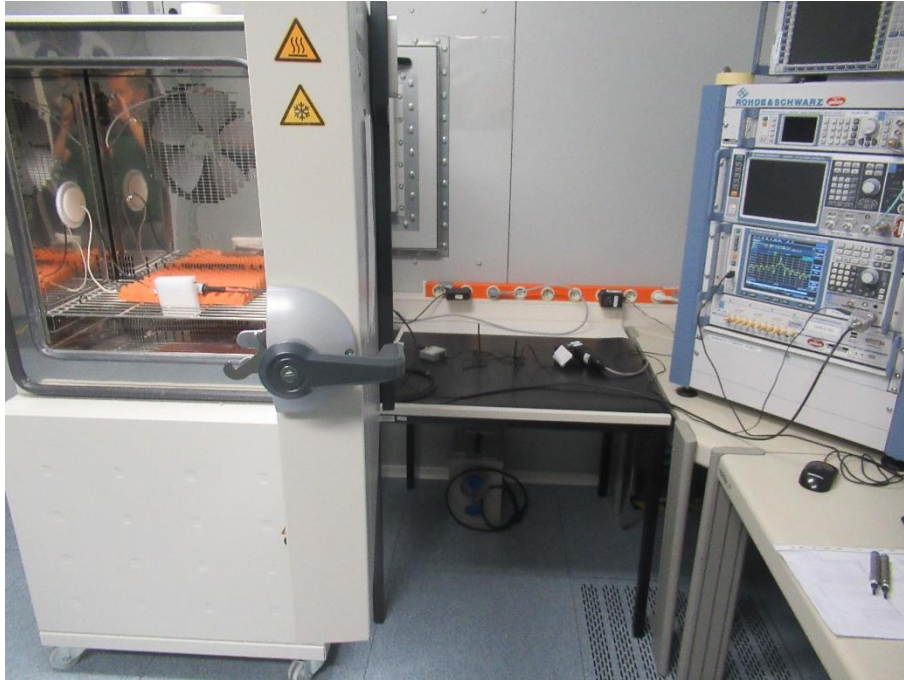
Photo 9 Bench test set up for (99% / 20 dB Bandwidth and Frequency Stability) (@ Ambient + Extreme Temperature, as required)
