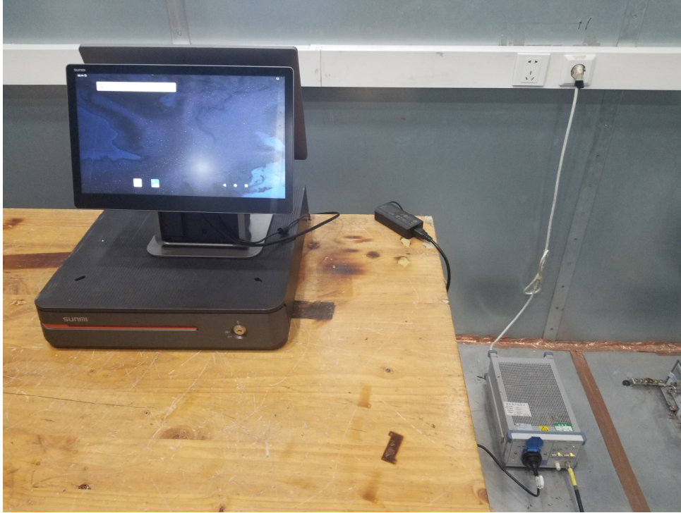
Picture 2: Conducted Emissions Test Setup
