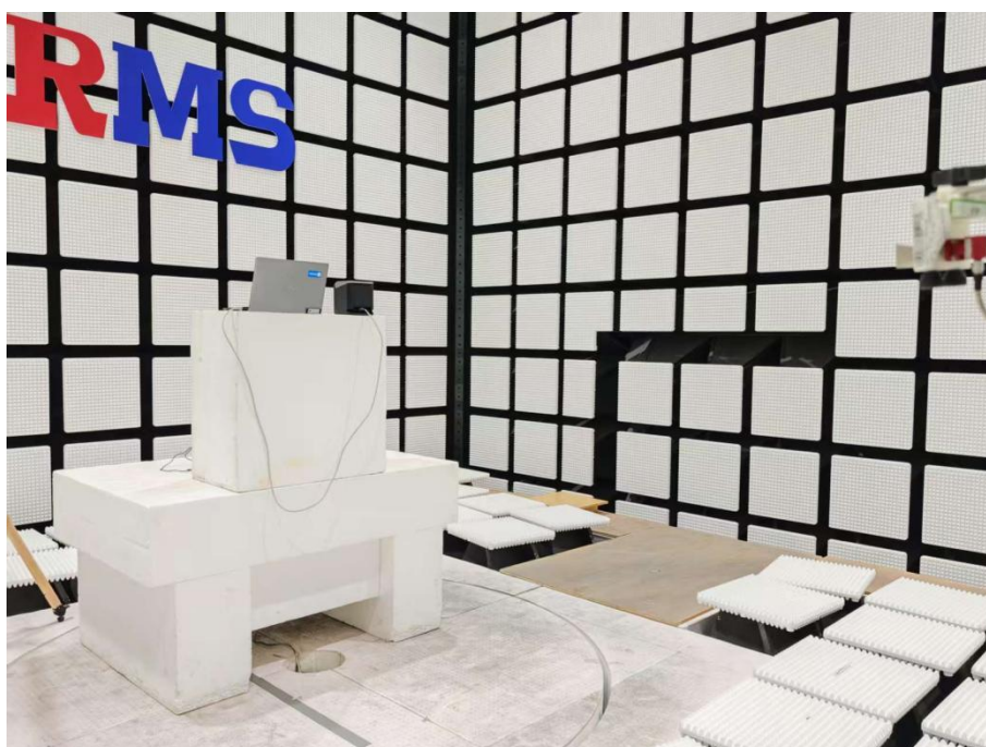
Description: Radiated Emission Test Setup (26.5GHz-40GHz)
