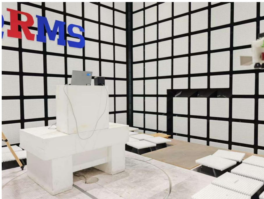
Description: Radiated Emission Test Setup (18GHz-26.5GHz)
