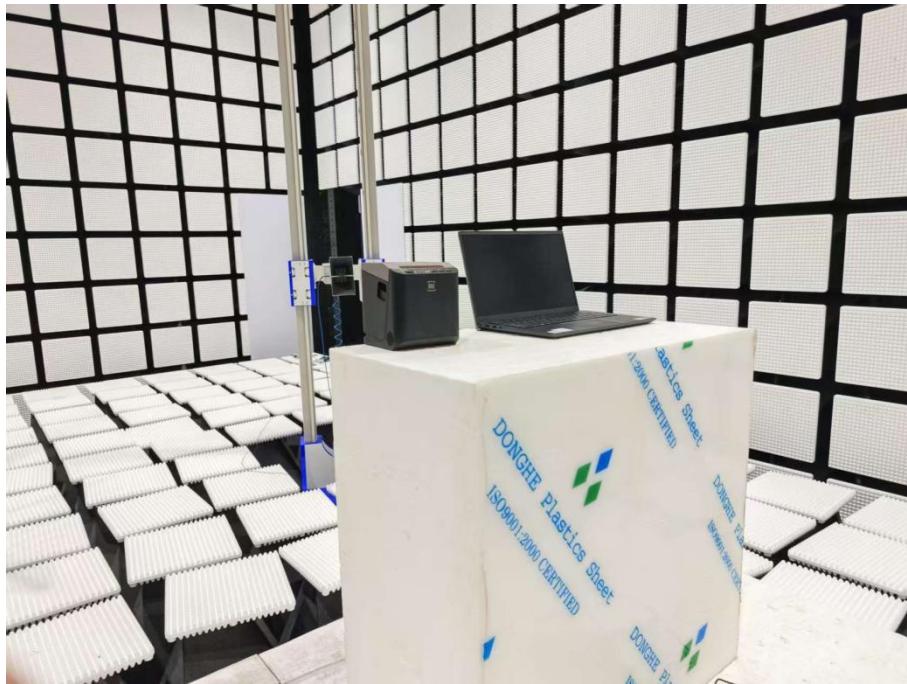
Description: Radiated Emission Test Setup (18GHz-26.5GHz)
