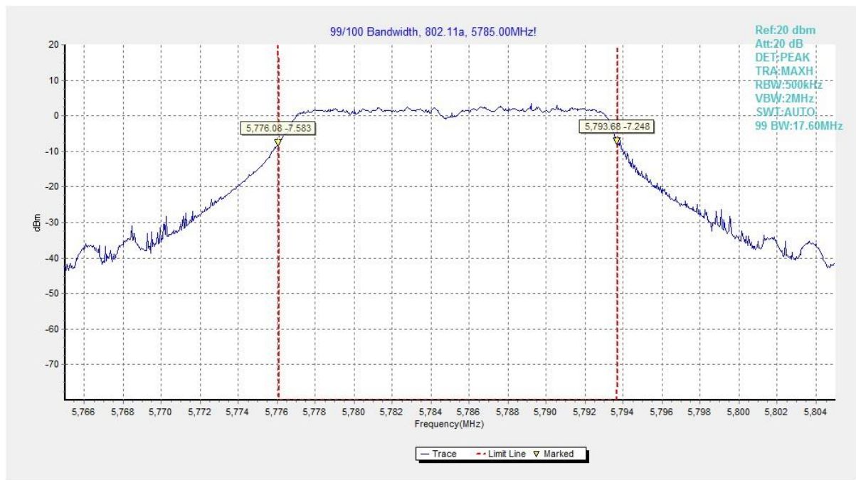
Fig. 35 99% Occupied Bandwidth (802.11a, 5785MHz)
