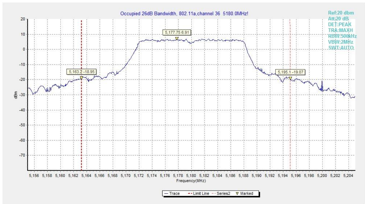
Fig. 1 Occupied 26dB Bandwidth (802.11a, 5180MHz)
