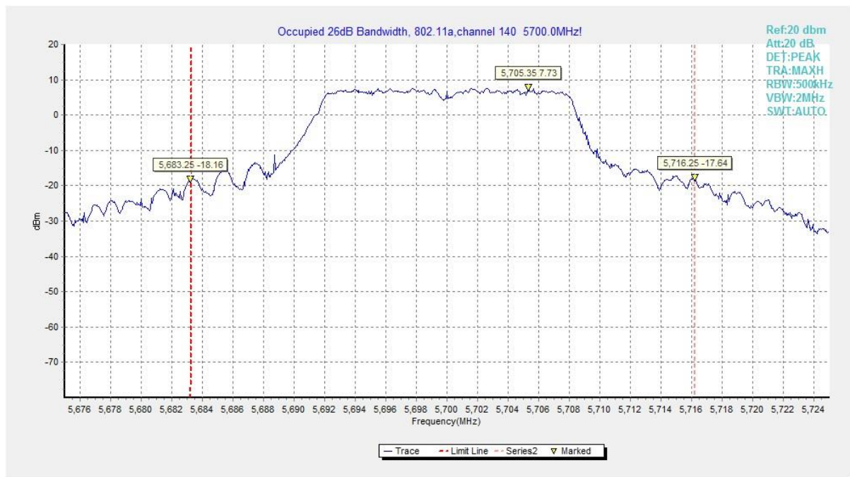
Fig. 9 Occupied 26dB Bandwidth (802.11a, 5700MHz)
