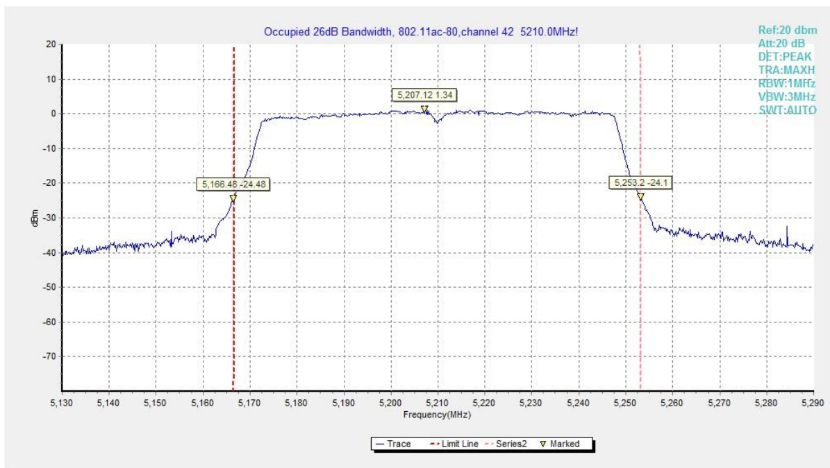
Fig. 16 Occupied 26dB Bandwidth (802.11ac-VHT80, 5210MHz)
