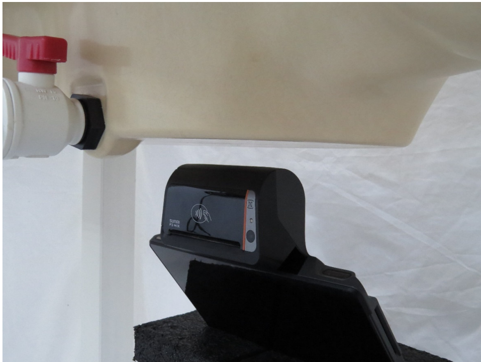
Picture 10: Main Antenna Top Edge, the distance from EUT to the bottom of the Phantom is 19mm
