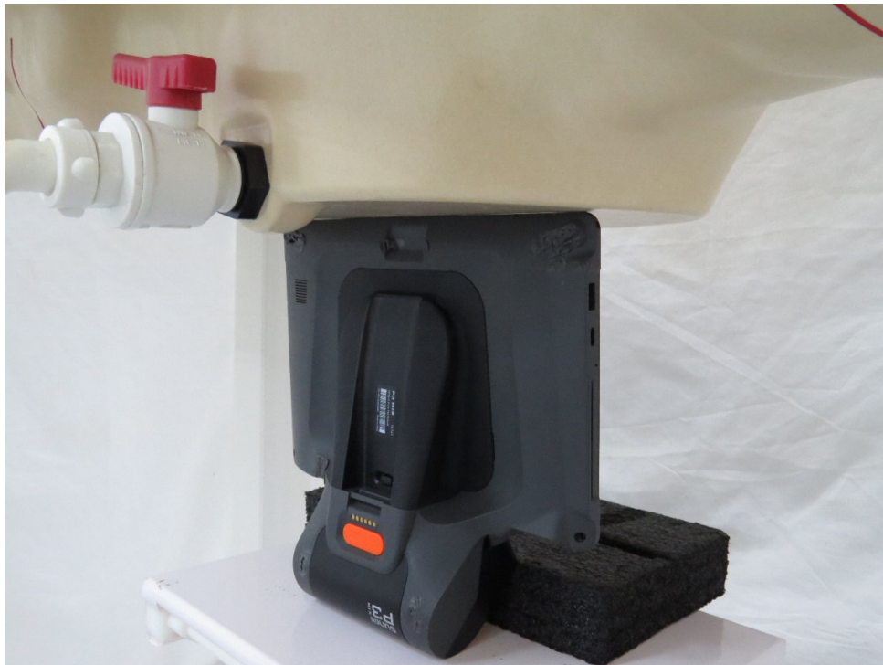
Picture 16: Hyper Wi-Fi Antenna Bottom Edge, the distance from EUT to the bottom of the Phantom is 0mm
