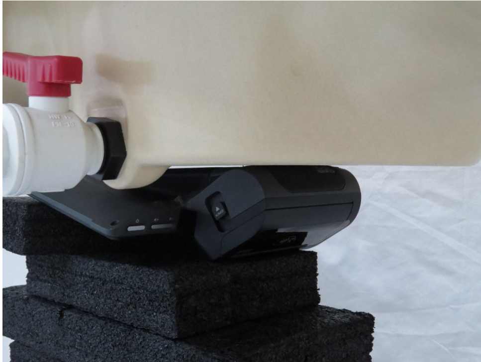
Picture 1: Main Antenna Back Side, the distance from EUT to the bottom of the Phantom is 0mm
