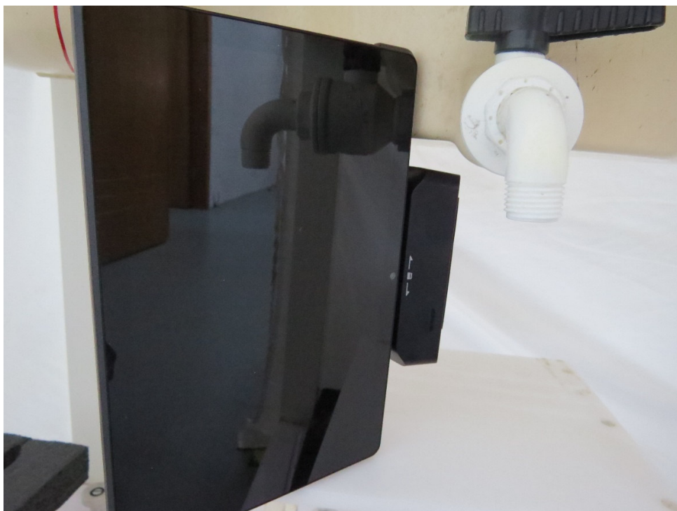
Picture 6: Main Antenna Left Edge, the distance from EUT to the bottom of the Phantom is 19mm
