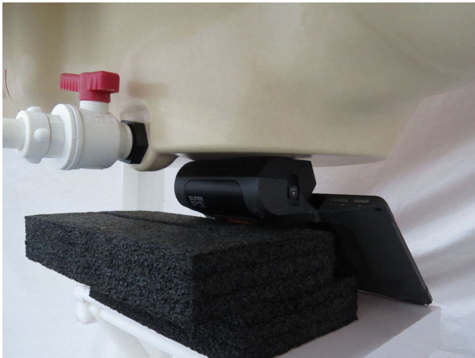
Picture 3: Main Antenna Front Side, the distance from EUT to the bottom of the Phantom is 0mm
