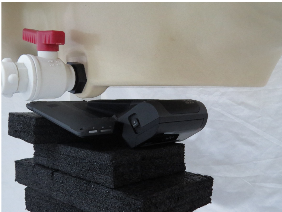
Picture 2: Main Antenna Back Side, the distance from EUT to the bottom of the Phantom is 19mm
