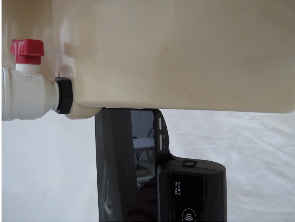
Picture 15: Hyper Wi-Fi Antenna Left Edge, the distance from EUT to the bottom of the Phantom is 0mm
