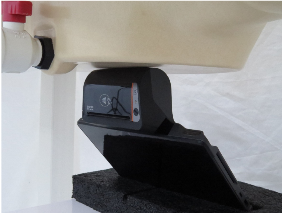
Picture 9: Main Antenna Top Edge, the distance from EUT to the bottom of the Phantom is 0mm
