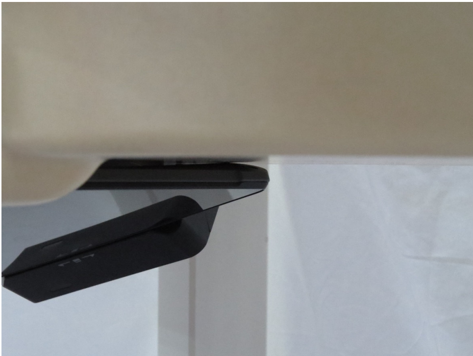
Picture 14: Hyper Wi-Fi Antenna Back Side, the distance from EUT to the bottom of the Phantom is 0mm
