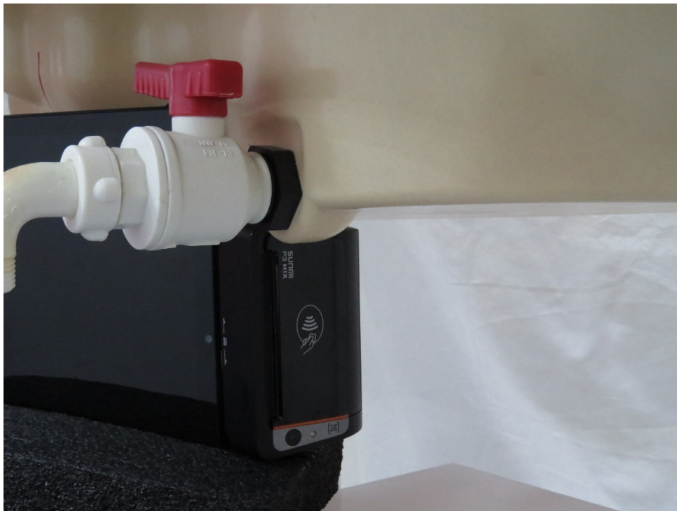
Picture 5: Main Antenna Left Edge, the distance from EUT to the bottom of the Phantom is 0mm
