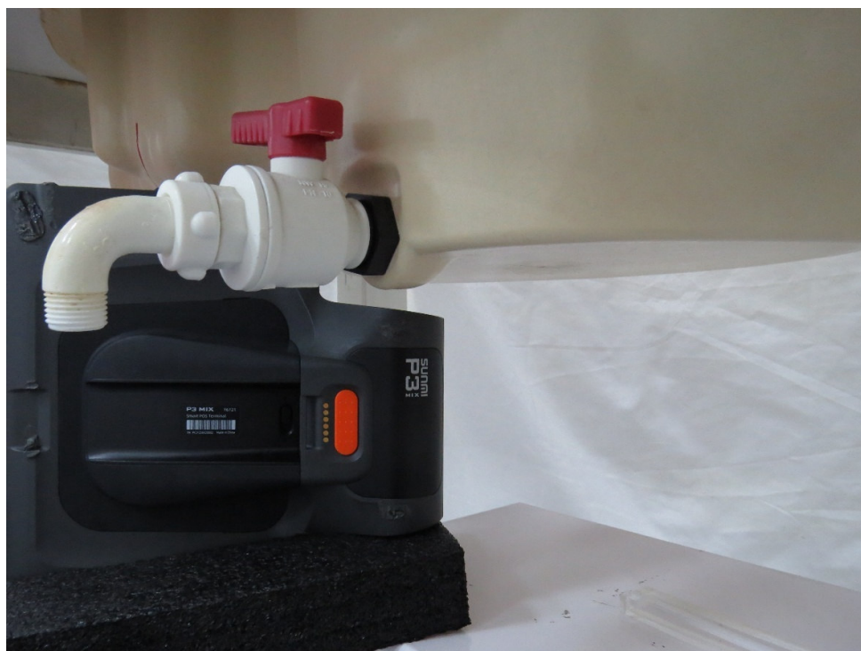
Picture 8: Main Antenna Right Edge, the distance from EUT to the bottom of the Phantom is 19mm
