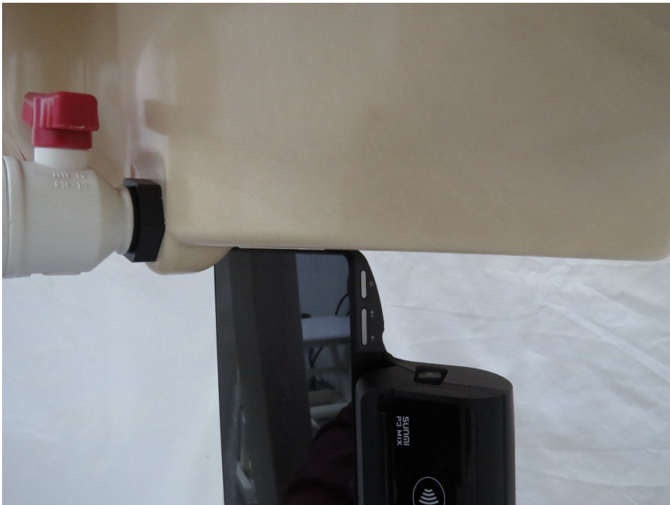
Picture 12: WLAN Antenna Left Edge, the distance from EUT to the bottom of the Phantom is 0mm
