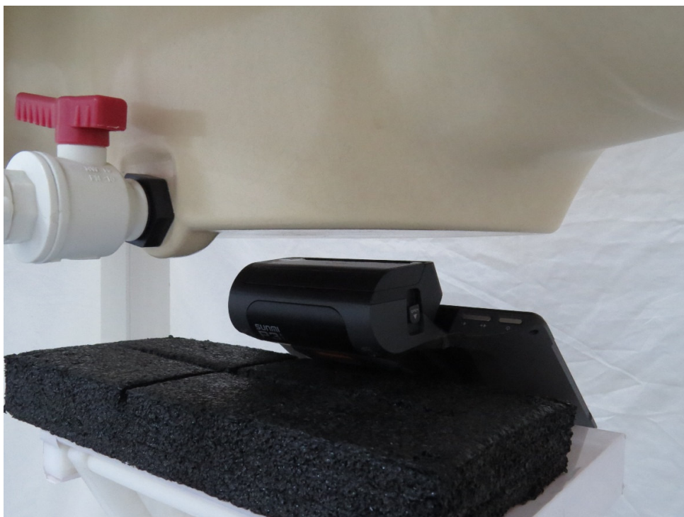
Picture 4: Main Antenna Front Side, the distance from EUT to the bottom of the Phantom is 19mm
