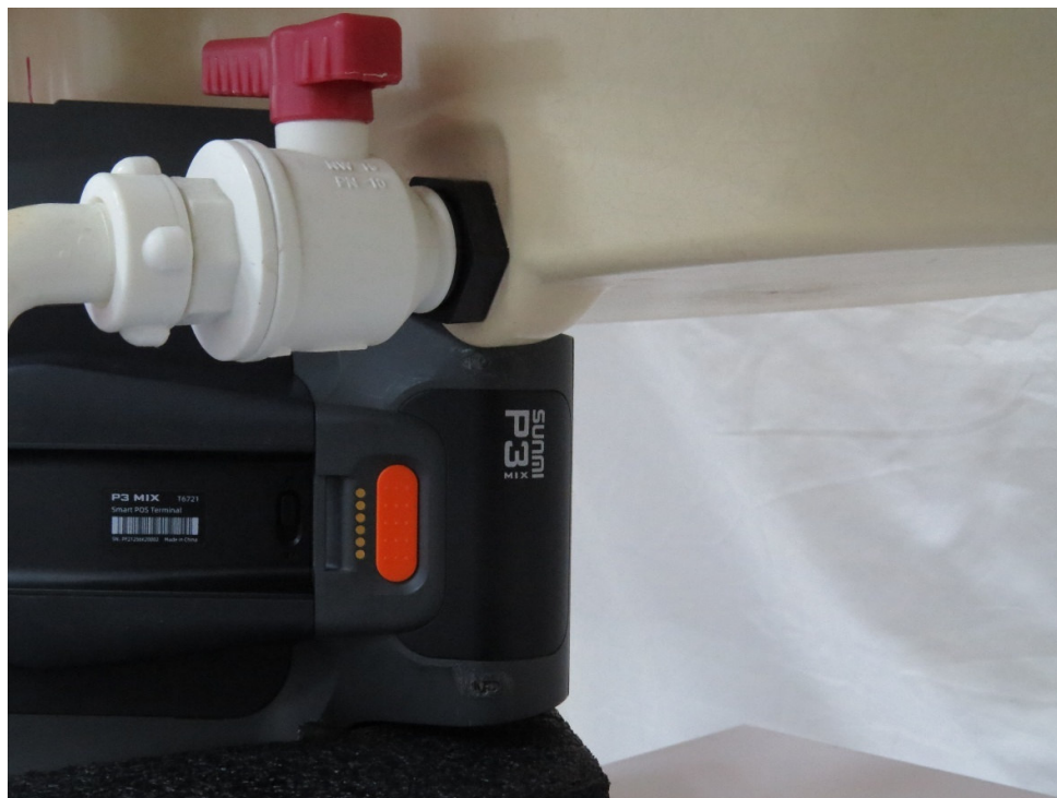
Picture 7: Main Antenna Right Edge, the distance from EUT to the bottom of the Phantom is 0mm
