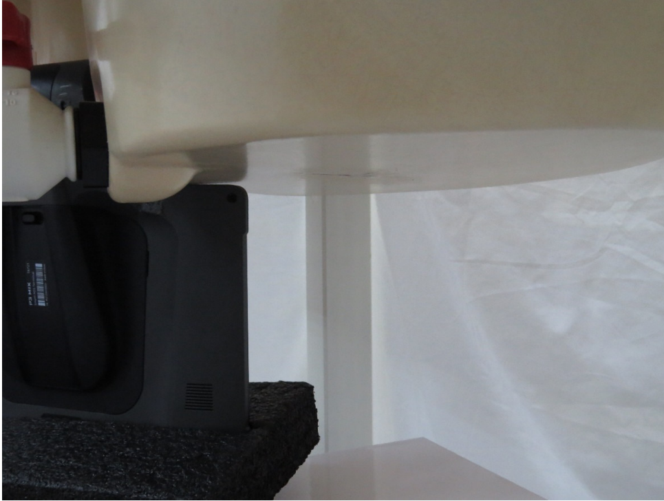
Picture 13: WLAN Antenna Top Edge, the distance from EUT to the bottom of the Phantom is 0mm
