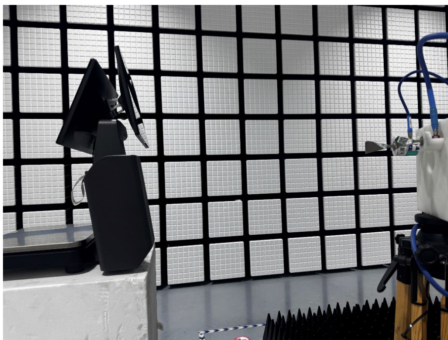
Description: Radiated Emission Test Setup (Above 18GHz)
