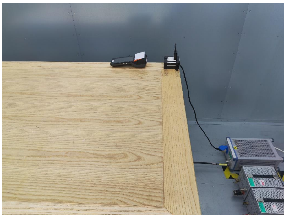
Description: Conducted Emission Test Setup
