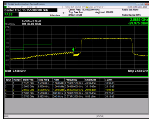
Band38 QPSK BW=10MHz LowChannel=37800 RB Size=50 Position=#0
