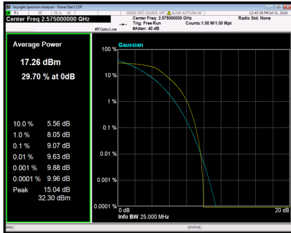
Band38 QPSK BW=10MHz Channel=37800 RB Size=50 Position=#0
