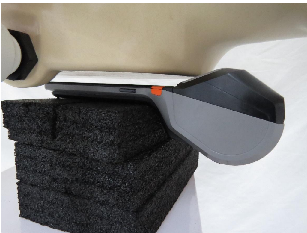
Picture 4: WLAN Antenna Front Side, the distance from EUT to the bottom of the Phantom is 10mm
