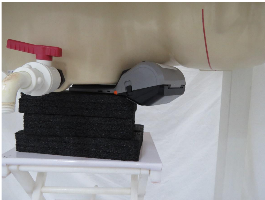
Picture 11: WLAN Antenna Back Side, the distance from EUT to the bottom of the Phantom is 0mm
