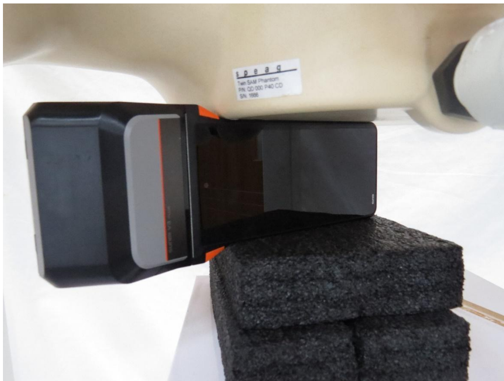
Picture 17: WLAN Antenna Right Edge, the distance from EUT to the bottom of the Phantom is 0mm
