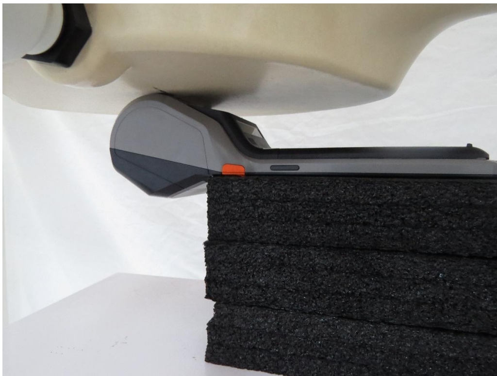
Picture 10: Mian Antenna Back Side, the distance from EUT to the bottom of the Phantom is 0mm
