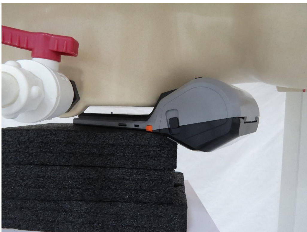
Picture 2: WLAN Antenna Back Side, the distance from EUT to the bottom of the Phantom is 10mm
