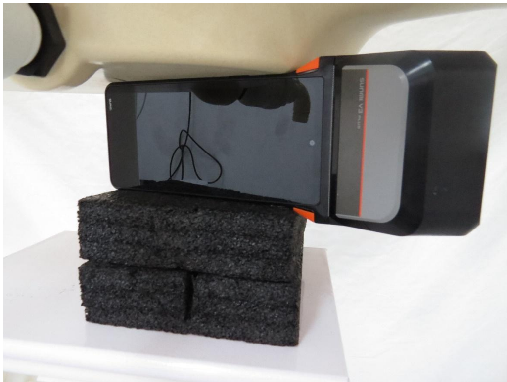
Picture 15: WLAN Antenna Left Edge, the distance from EUT to the bottom of the Phantom is 0mm
