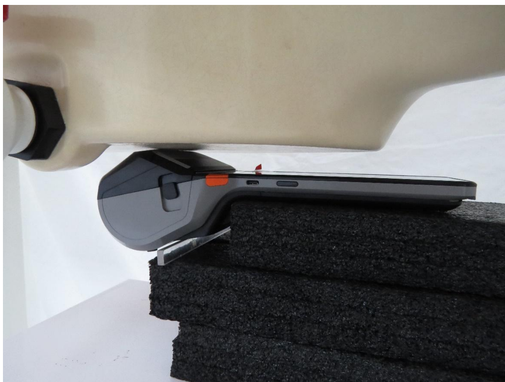
Picture 12: Mian Antenna Front Side, the distance from EUT to the bottom of the Phantom is 0mm
