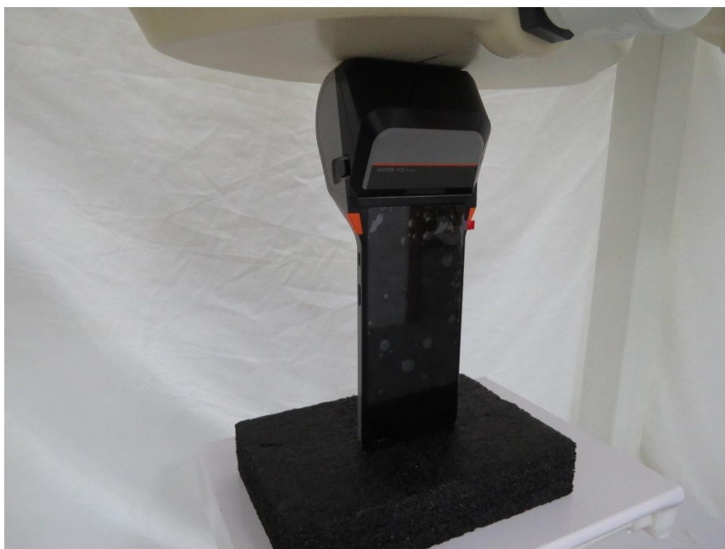
Picture 18: Mian Antenna Top Edge, the distance from EUT to the bottom of the Phantom is 0mm
