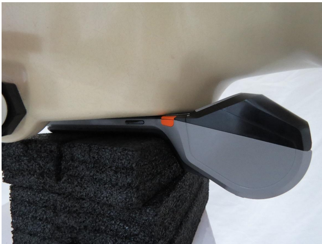
Picture 13: WLAN Antenna Front Side, the distance from EUT to the bottom of the Phantom is 0mm
