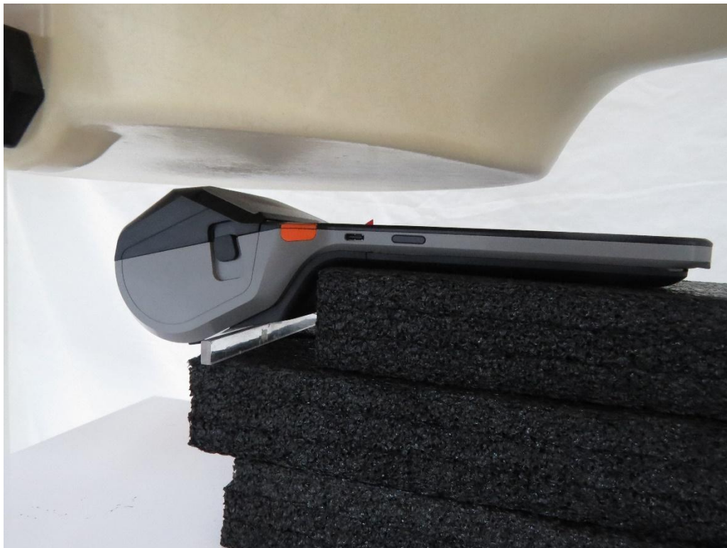
Picture 3: Mian Antenna Front Side, the distance from EUT to the bottom of the Phantom is 10mm
