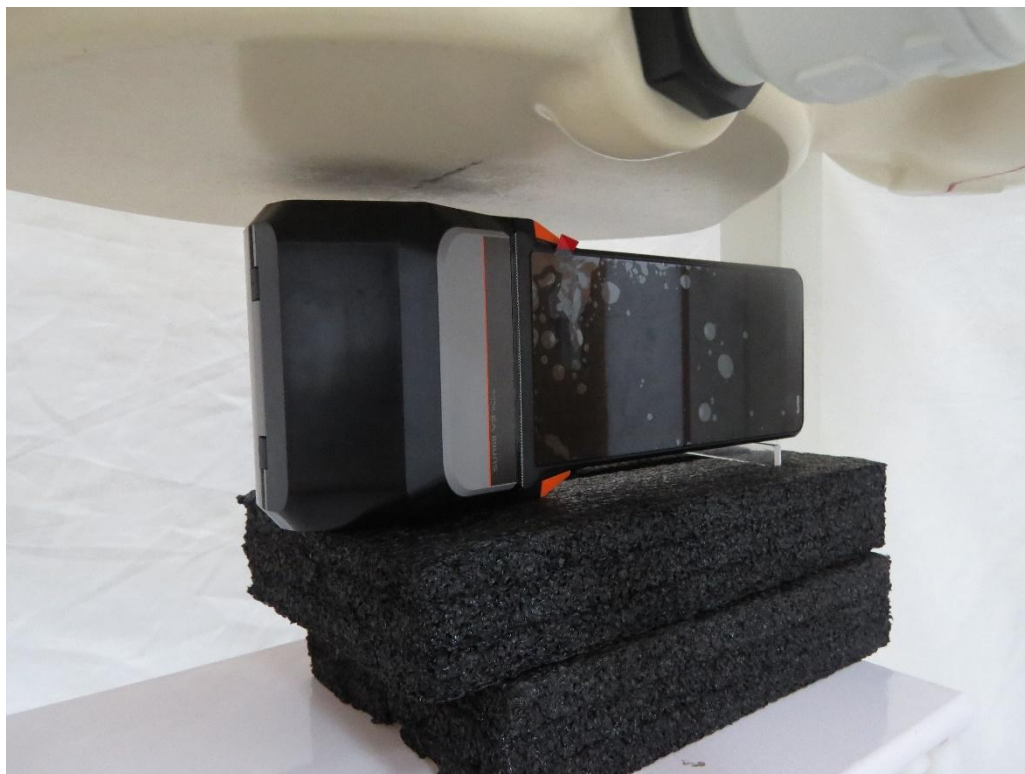
Picture 7: Mian Antenna Right Edge, the distance from EUT to the bottom of the Phantom is 10mm
