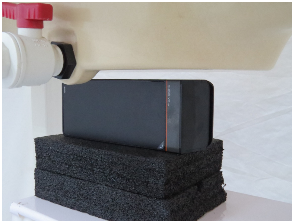
Picture 5: Left Edge, the distance from EUT to the bottom of the Phantom is 10mm
