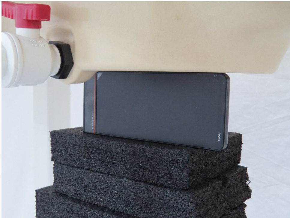
Picture 10: Right Edge, the distance from EUT to the bottom of the Phantom is 0mm
