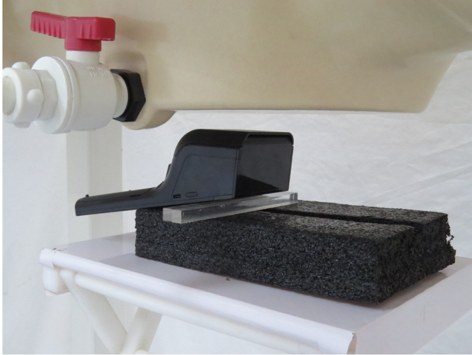
Picture 11: Back Side, the distance from EUT to the bottom of the Phantom is 14mm
