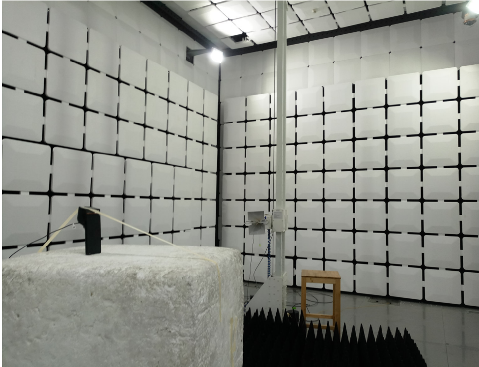
Picture 1 Radiated Emission Test Setup
