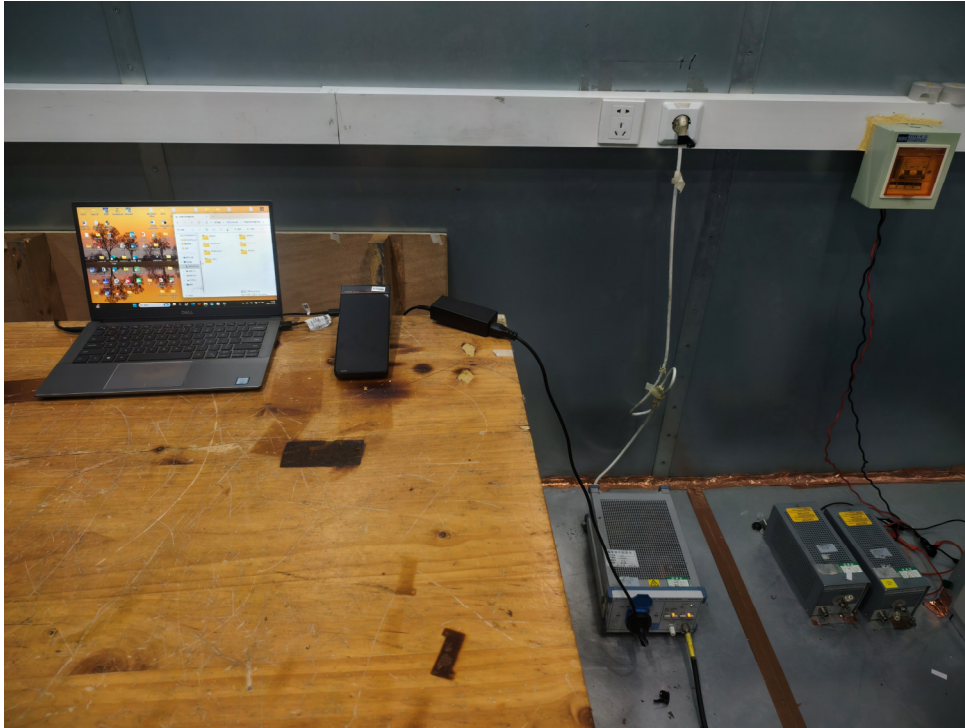
Picture 2: Conducted Emissions Test Setup
