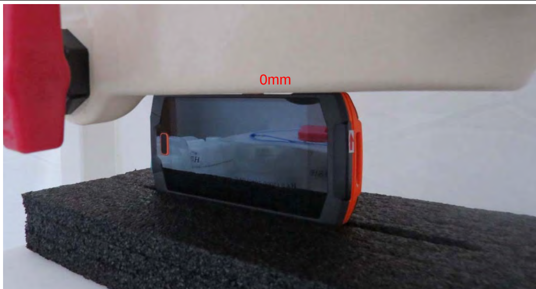
Picture 7: Left Side, the distance from handset to the bottom of the Phantom is 0mm
