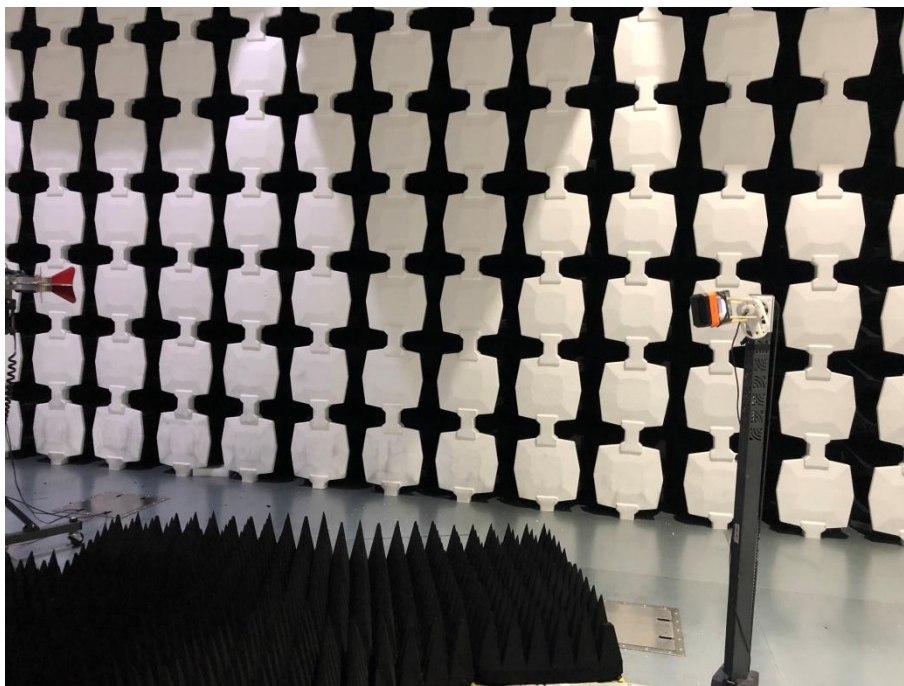
Description: Substitution Antenna for EIRP Test
