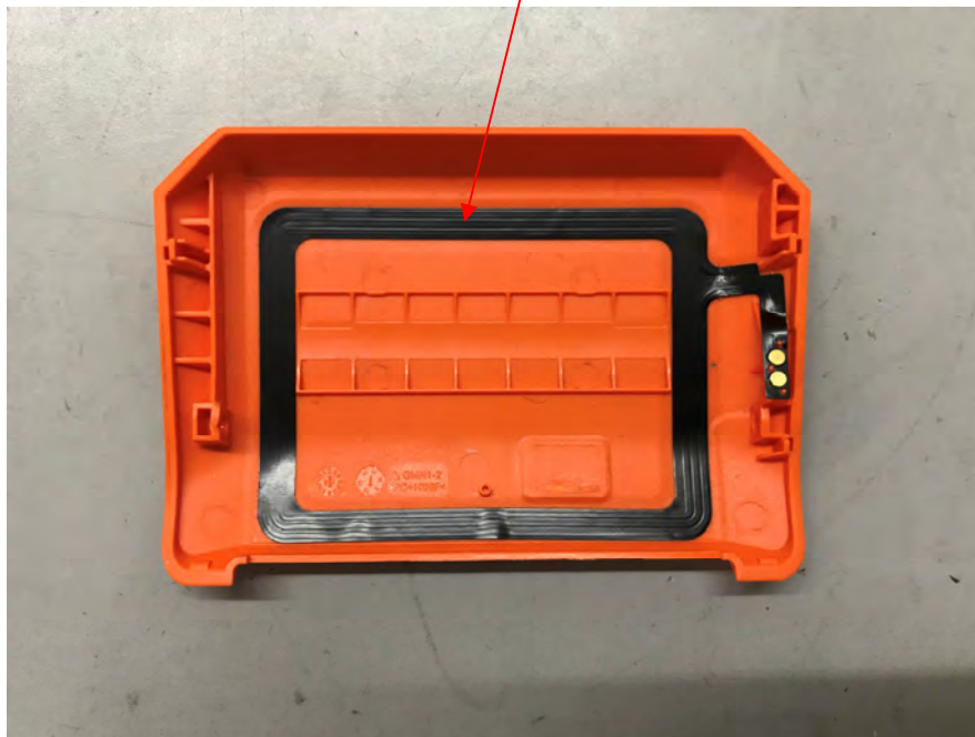
EUT – NFC Antenna View
