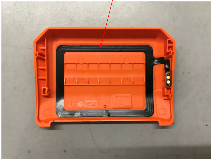
EUT – NFC Antenna View
