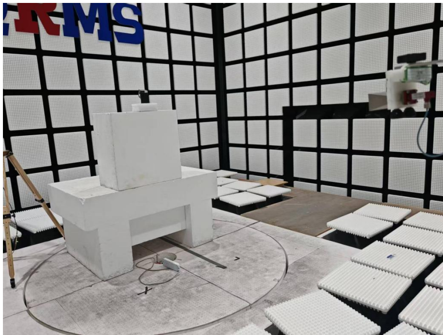
Description: Radiated Emission Test Setup (Above 18GHz)
