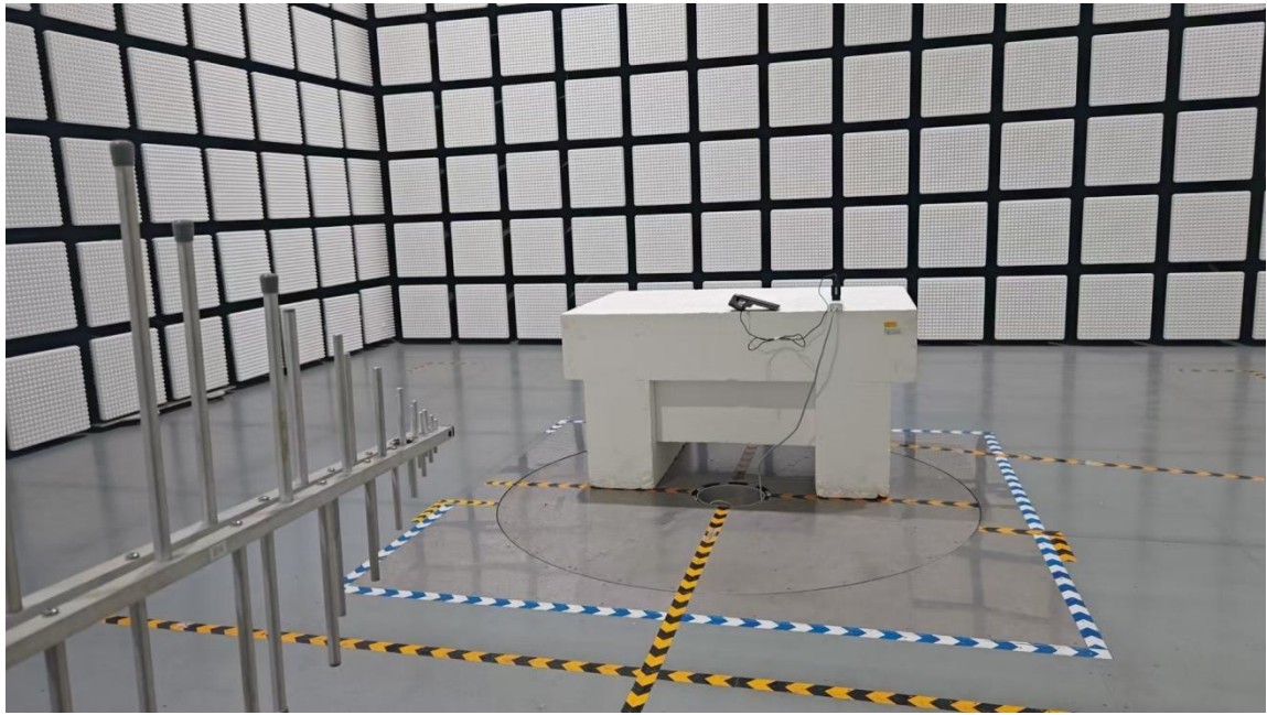
Description: Back view of Radiated Emission Test Setup (Below 1GHz)
