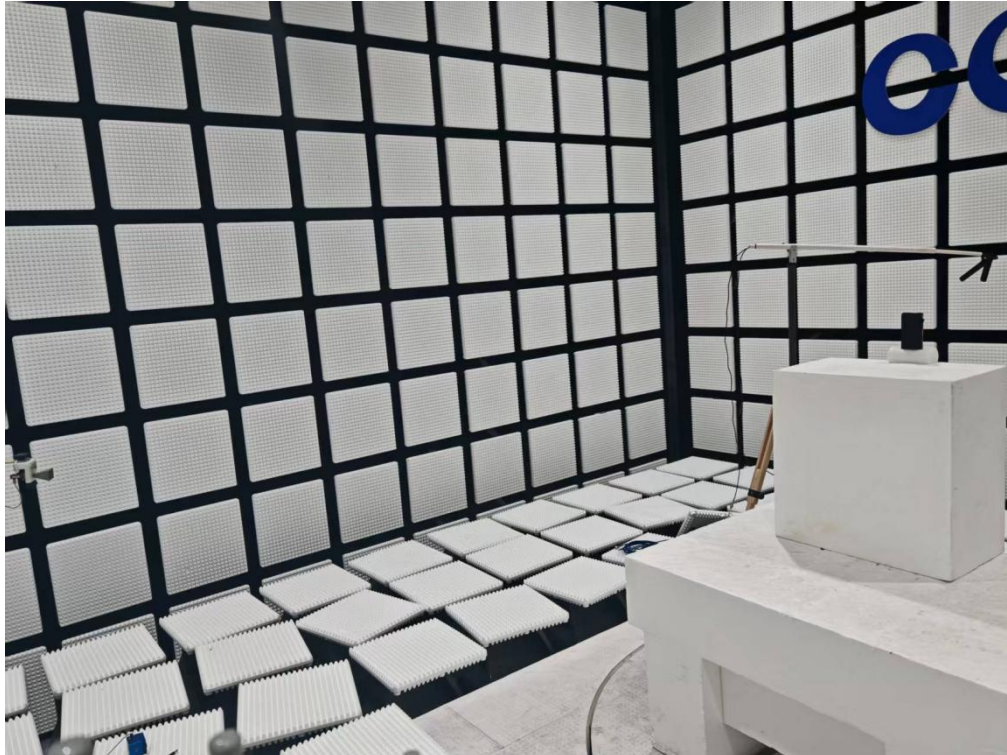
Description: Radiated Emission Test Setup (18GHz -26.5GHz)
