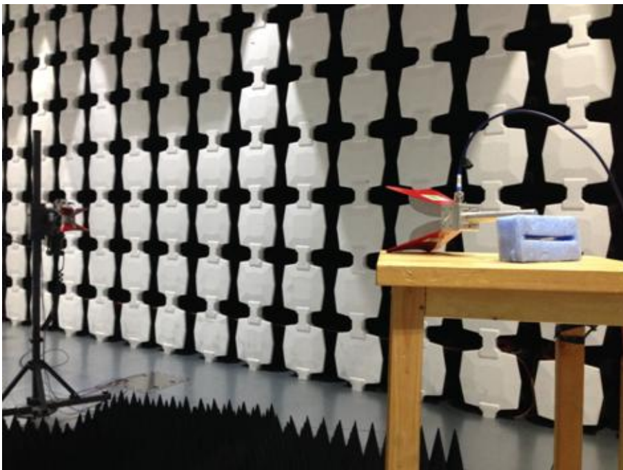
Description: Substitution Antenna for EIRP Test
