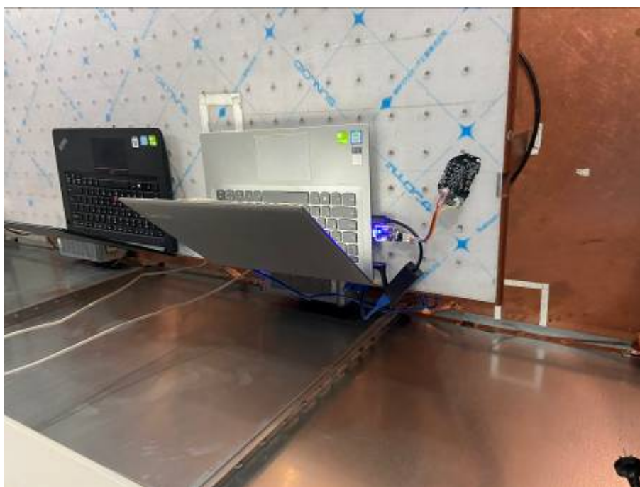
Conducted Emissions Test Setup (with laptop)
