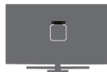
Fix the bracket to the back of the monitor with screws.
