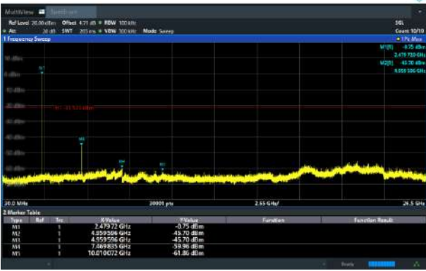
GFSK on Channel 78
