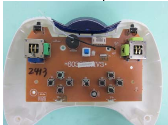
Inner Circuit Top View
