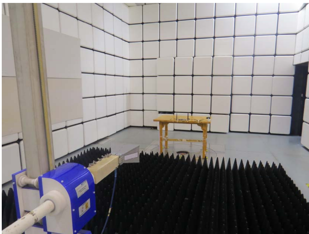
Picture 2: Radiated Spurious Emissions Test setup
