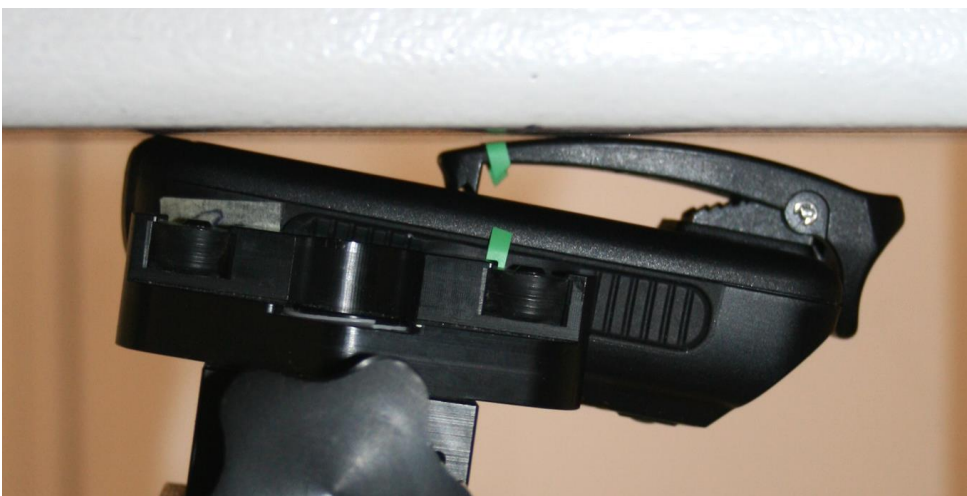
Test position "Back".DUT with back side towards the phantom with 0mm separation
