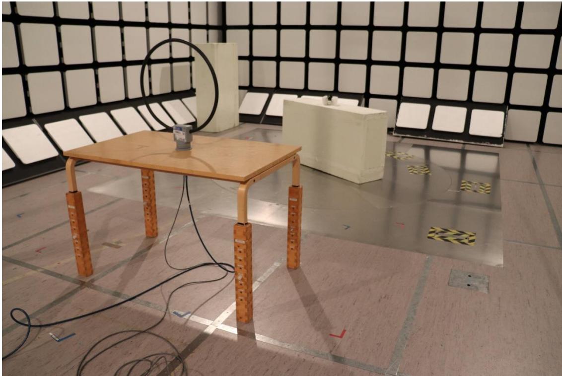
Photograph 1. Radiated Spurious Emissions 0.009 - 30 MHz
