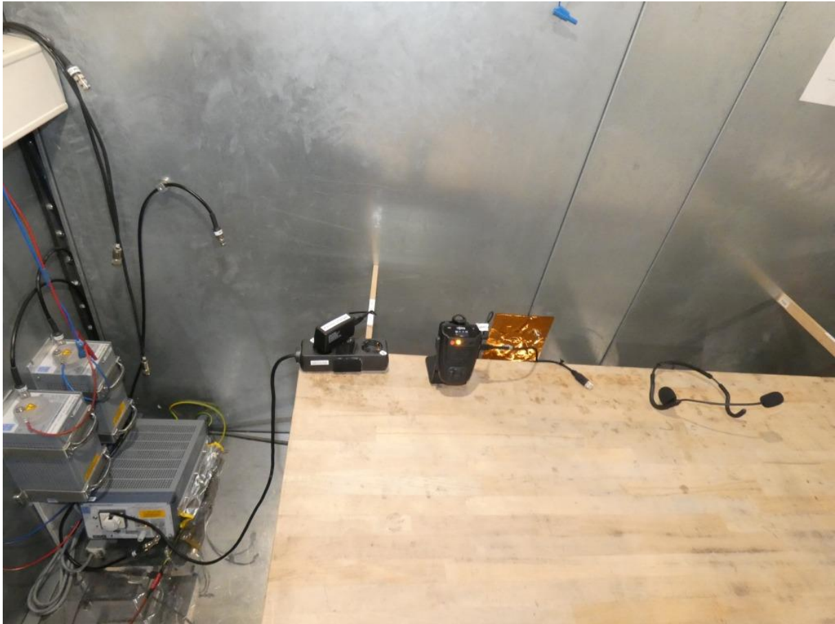
Photo 2: Test setup for conducted measurements (Test Setup: stand alone, AC mains connection: connected via docking station, unintentional radiator §15.107, ANSI C63.4)
