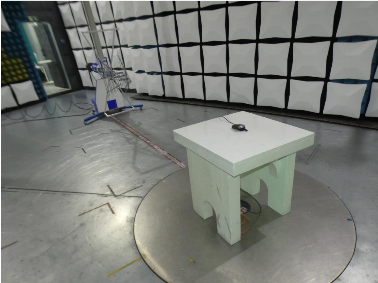
Photo 6: Test setup for radiated measurements (stand alone setup, 30 MHz - 1 GHz; FCC 15c247)
