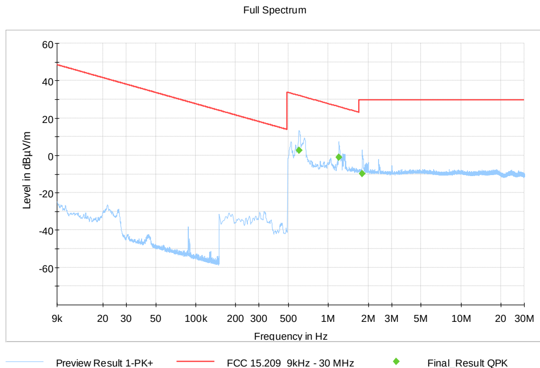
Figure 74: Unwanted Emissions, radiated 9 kHz – 30 MHz (1 Mbps, TX 2480 MHz)
