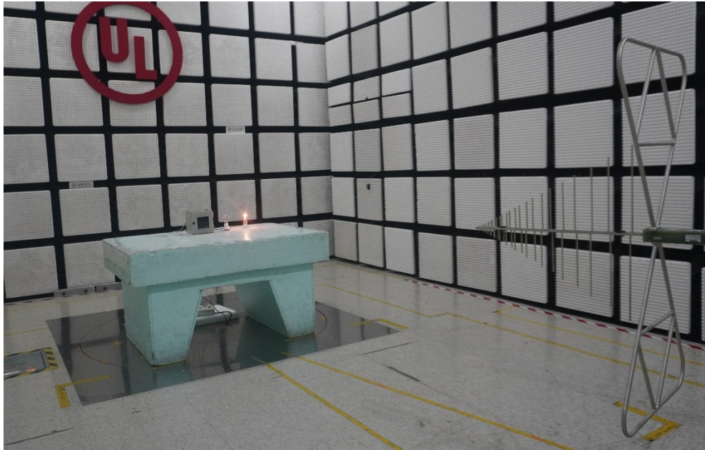
Radiated Emission_30MHz to 1 GHz_Vertical Polarization
